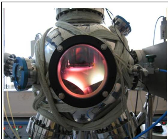
**Figure 2.6: Photograph of the sputtering unit at SSPD, BARC during deposition.**
