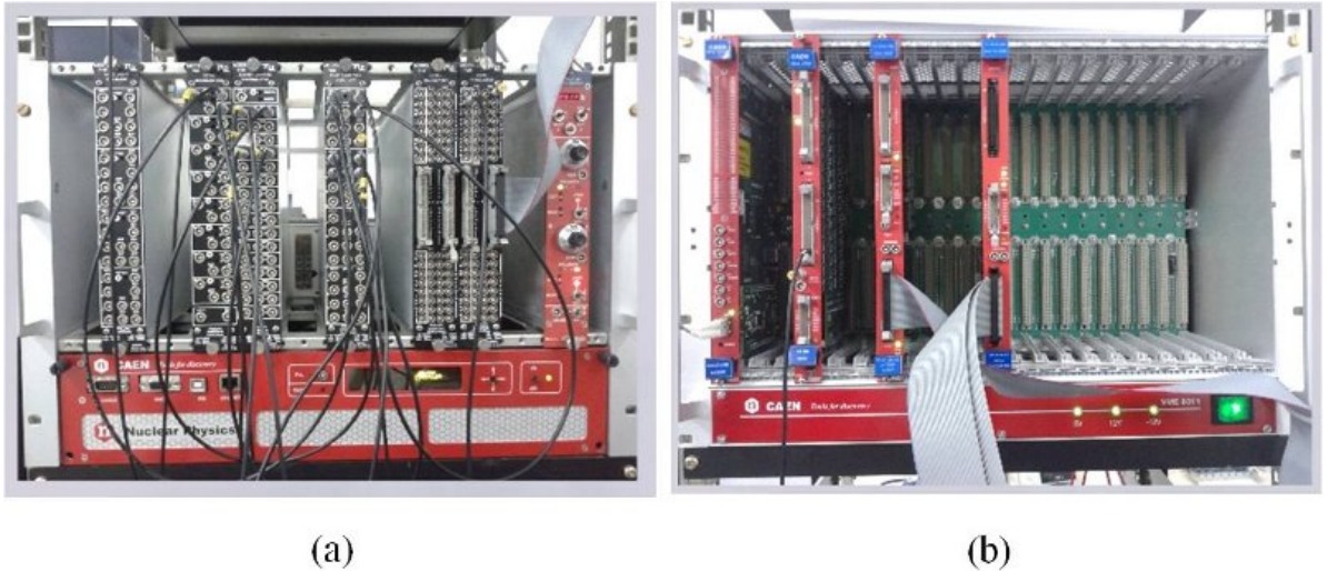
Figure 5.13: (a) NIM and (b) VME-based data acquisition system.
