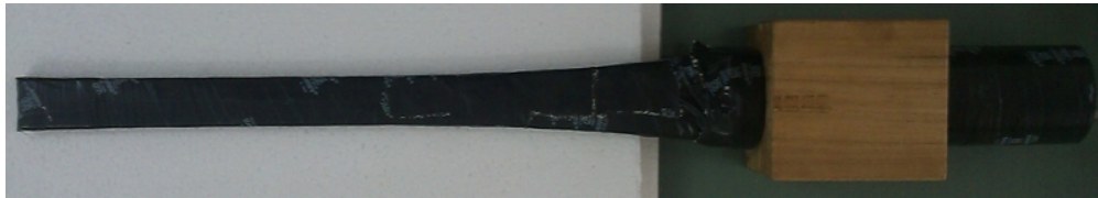
Figure 4.11: A 30 \times 3 \times 1 \text{ cm}^3 cosmic-ray paddle.
