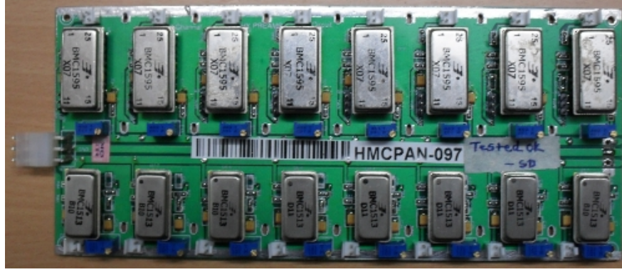
Figure 5.12: A 8-in-1 two-stage Hybrid Micro Circuit (HMC) based high speed preamplifier board.
