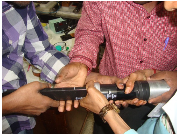
Figure 4.10: Assembly of cosmic-ray paddle.
