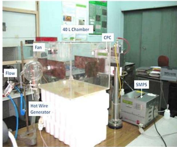
Fig. 6.1 (b): Experimental arrangement in 40 L chamber
