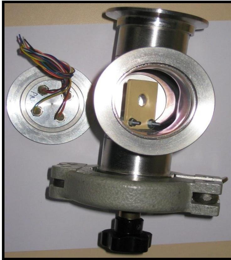
**Figure 3.21.** Detector mounting jig with goniometer.
