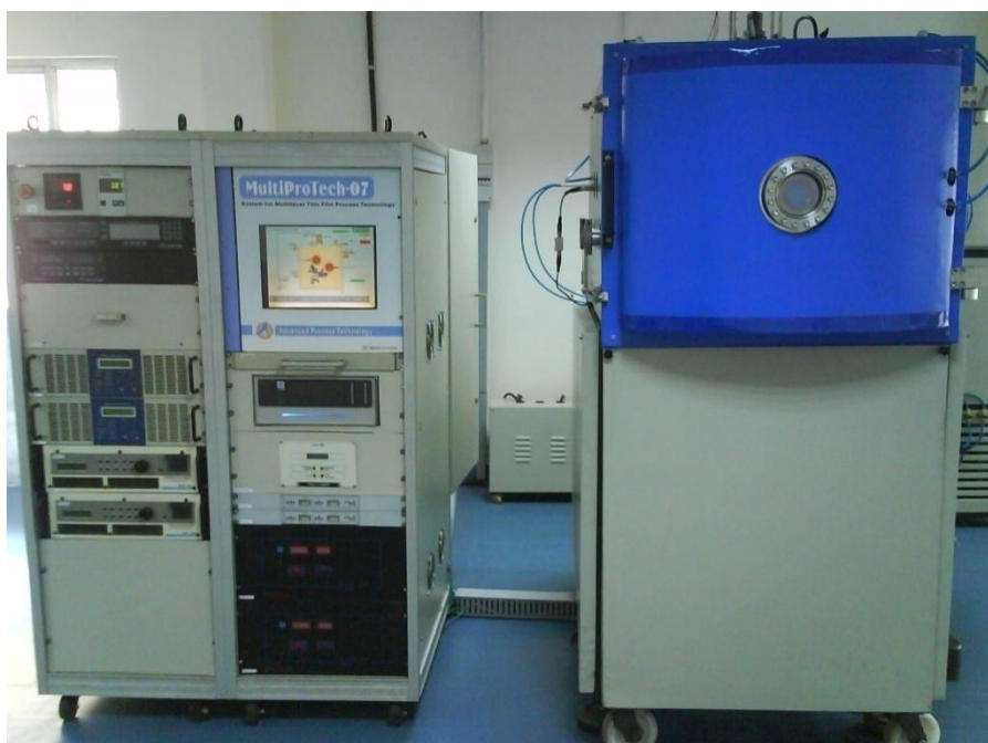
Fig. 2.10: Custom Made DC/RF/Pulse DC Magnetron Sputtering System at AMPD, BARC-Visakhapatnam Laboratory
