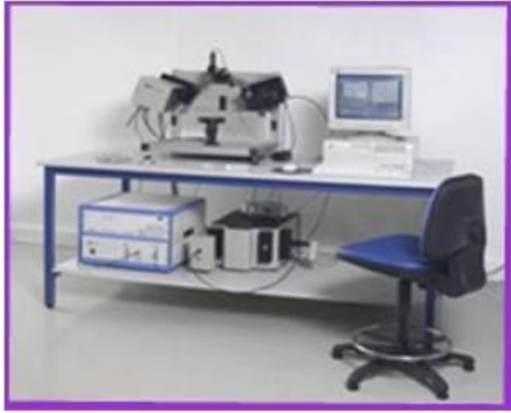
Fig. 2.25: Photograph of phase modulated spectroscopic ellipsometer at AMPD, BARC, Trombay
