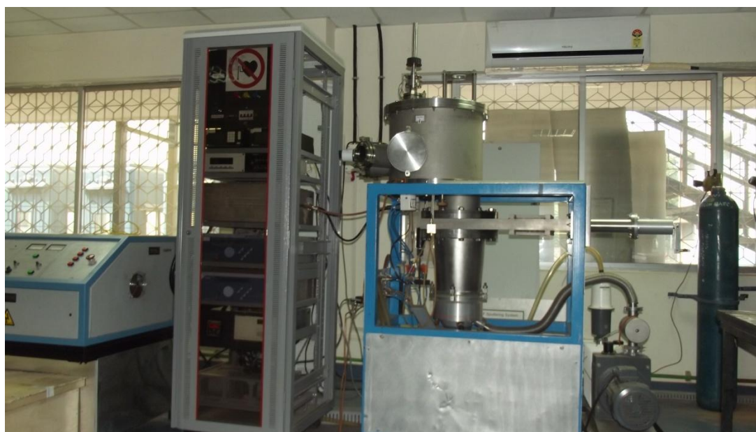
Fig. 2.9: In -house built DC/RF Magnetron Sputtering System at AMPD, BARC-Visakhapatnam Laboratory
