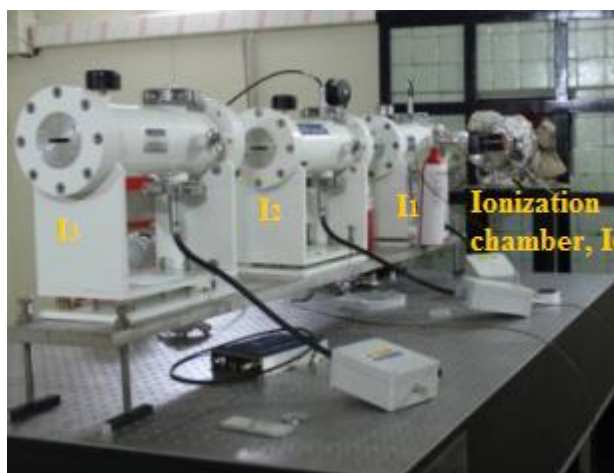
Fig. 2.45: Experimental set-up for transmission mode of XAFS measurement.
