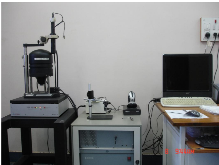
Fig. 2.27: Actual photograph of AFM set up located at Mechanical and Optical Support Section, RRCAT, India and used for AFM characterization of the samples in this thesis.
