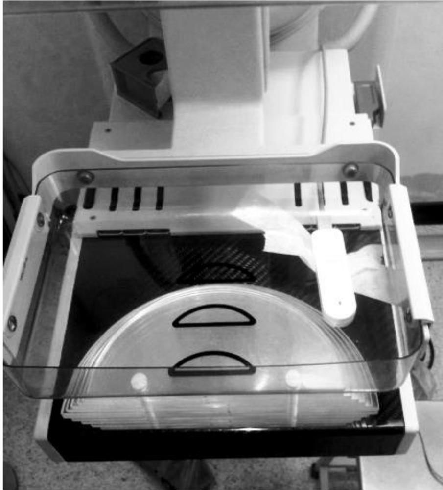
Figure 4.4 Experimental set up for measurement of breast entrance exposure (BEE) in mammography phantom
