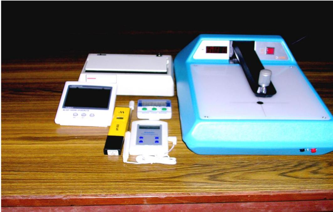
Figure 2.2 Photograph of processor quality control kit
