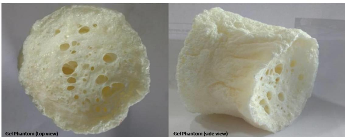
Figure 5.7 Top and side view of polymer gel phantom
