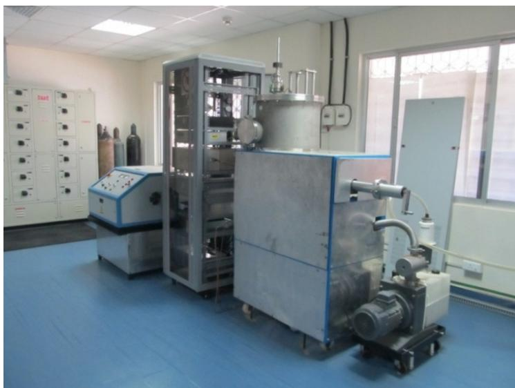
**Figure 2.3:** In-house built R.F. Magnetron sputtering deposition system at BARC-VIZAG, Visakapatnam.
