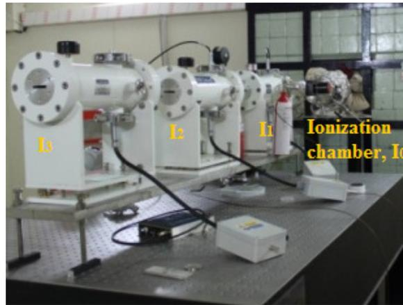
**Figure 2.13:** Experimental set-up for transmission mode of EXAFS measurement.
