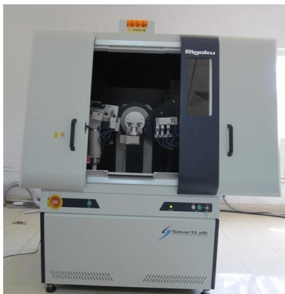
**Figure 2.26:** Rigaku SmartLab diffractometer used for experiment.
