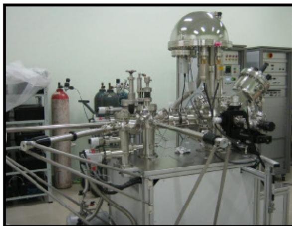
**Figure 2.33:** Photograph of XPS instrument.
