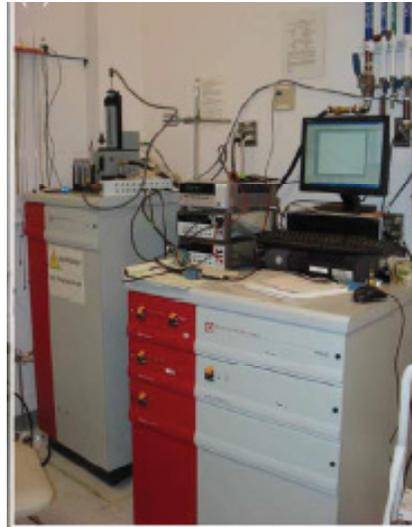
**Figure 2.34:** Photograph of SQUID-vibrating sample magnetometer.
