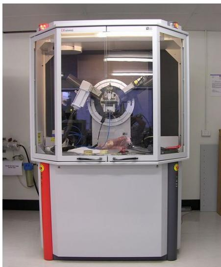
**Figure 2.25:** Bruker D8 Discover diffractometer used for experiment.
