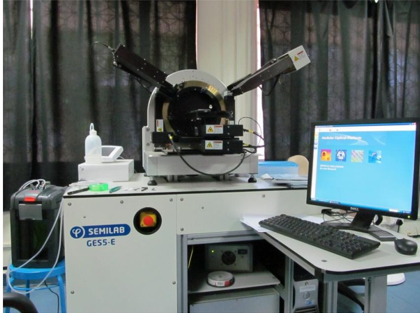
**Figure 2.28:** Photograph of spectroscopic ellipsometer (SOPRA GES5E)
