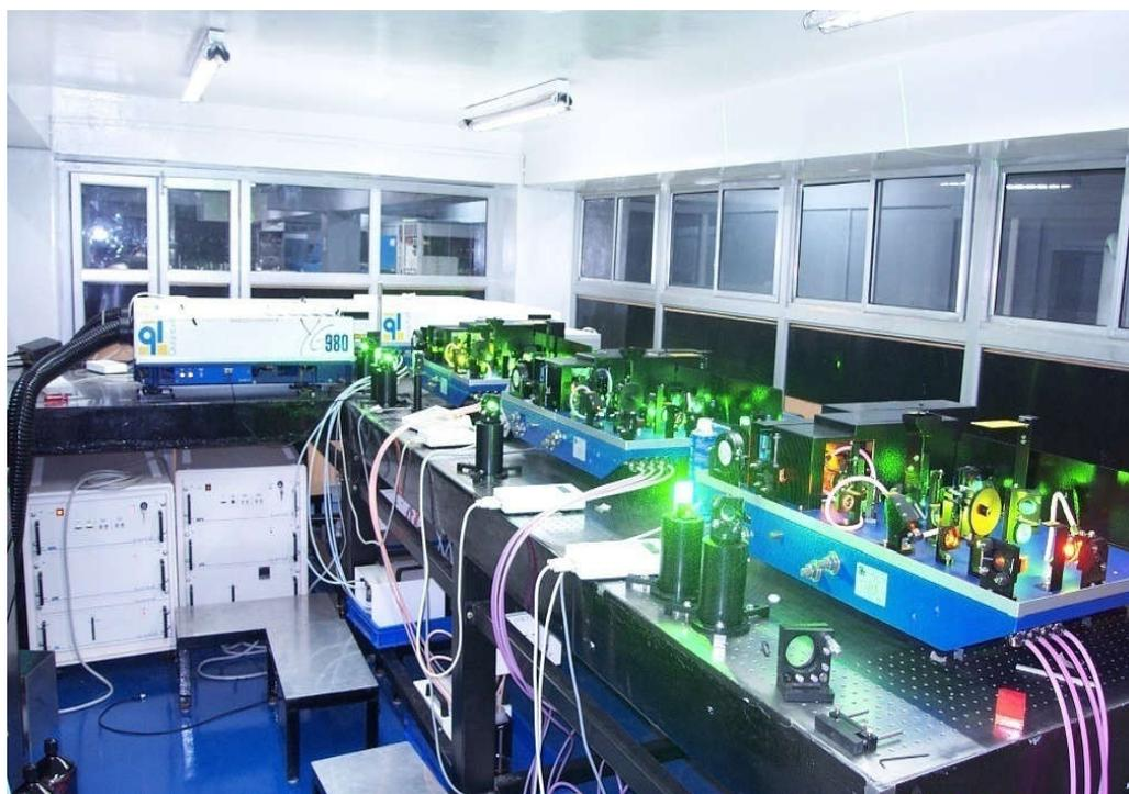
*Fig. 2.2: Laser systems used in photoionization experiments*
