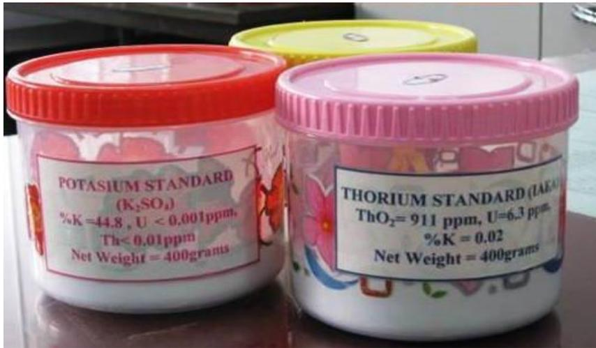
**Fig 2.9:** New Sample geometry: 5" dia,400 gms.
