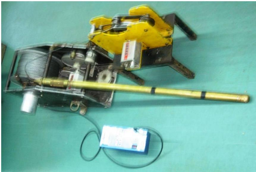
**Fig.2.11:** Gamma Ray logging system for exploratory boreholes.
