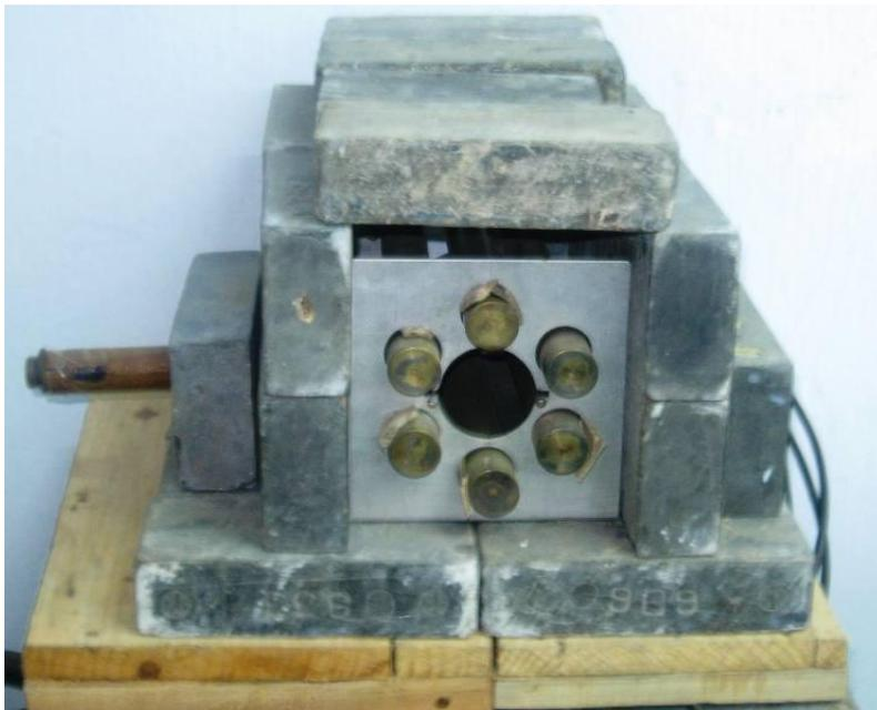
**Fig.2.2:** Core assay assembly using circular array of GM detectors.
