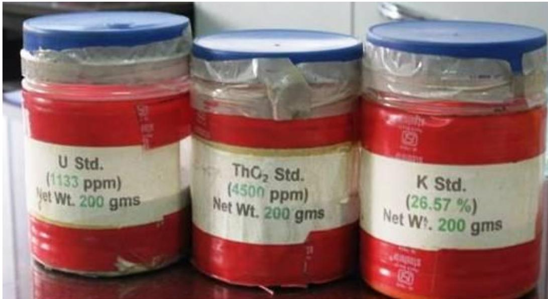
**Fig 2.7:** Old Sample geometry: 4" dia,200 gms.
