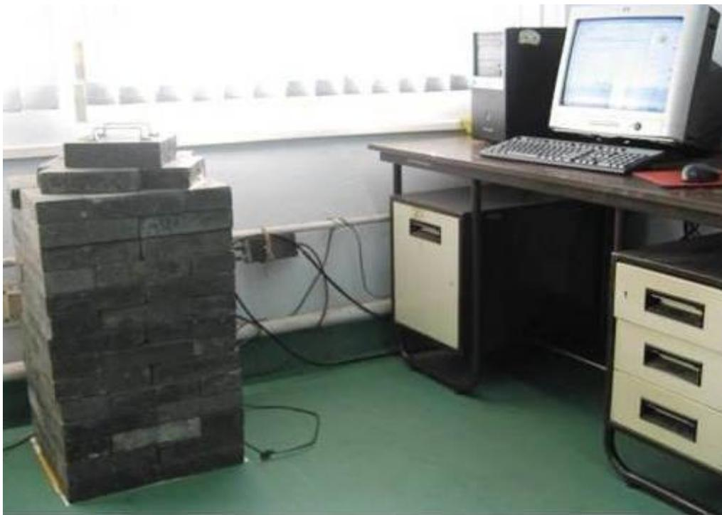
**Fig.2.5:** dMCA based Gamma ray spectrometer using 5"x4" NaI(Tl) detector.
