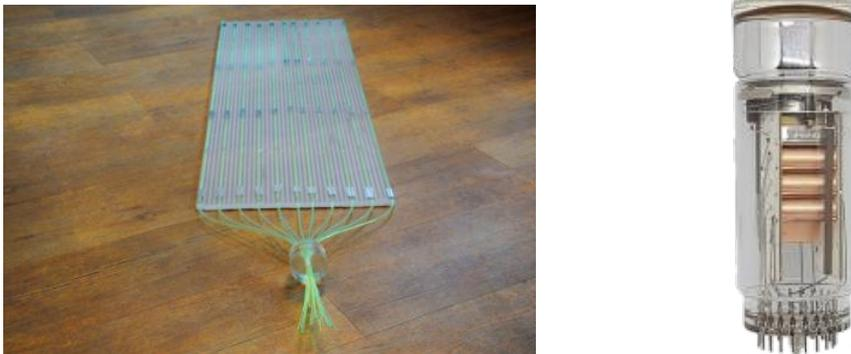
FIGURE 2.1: One of the 14 PSs with WLS fibres (left) and ET enterprises 9807B PMT (right)
