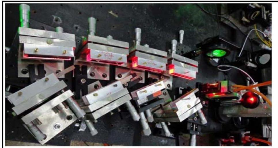
*Figure 4.21: Picture of the intra-cavity beam combined four wavelength laser system*
