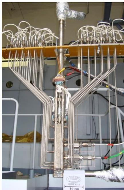
Figure 5.13: Photograph of the RF-test section in Experimental NaK loop at Efremov Institute, Russian Federation
