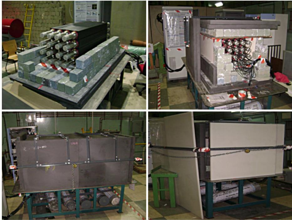
FIGURE 2.13: mini-ISMARAN 4×4 matrix with progressively increasing shielding in reactor environment.
