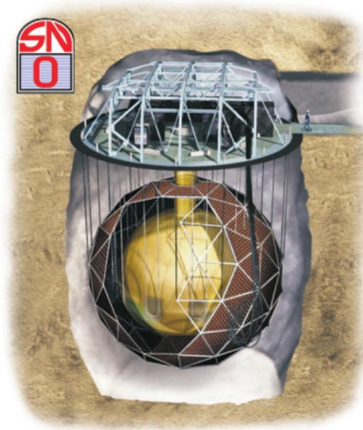
FIGURE 1.4: A schematic of Sudbury Neutrino Observatory 2039 m below the surface in a nickel mine near Sudbury, Ontario [31]
