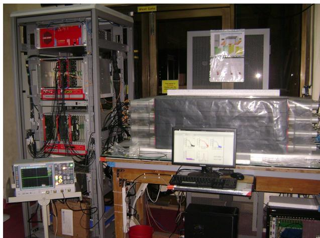
FIGURE 2.12: mini-ISMARAN 4×4 matrix in laboratory environment.
