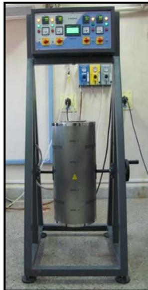
**Figure 2.5:** Photograph of the vertical Bridgman-Stockbarger crystal growth system used to grow CsI(Tl) single crystals [160], [161].
