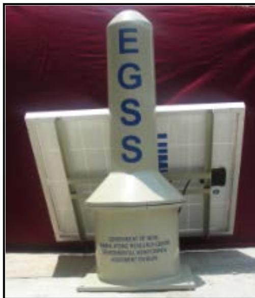
**Figure 6.4:** Photograph of EGSS (height: 92 cm, base area:  $35 \times 35 \text{ cm}^2$ , weight: 28 kg) [16].
