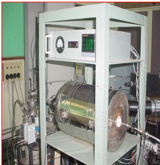
Figure 2.4: Photograph of the in house fabricated CVD system.
