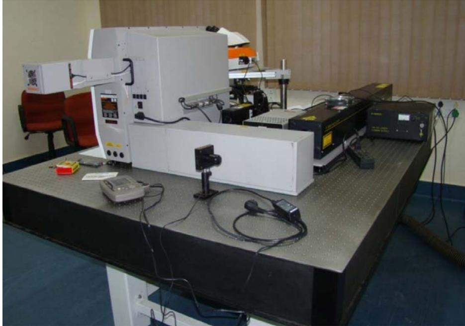
**Fig.2.10.** Renishaw *in-via* Raman spectrometer used for the Raman measurements.
