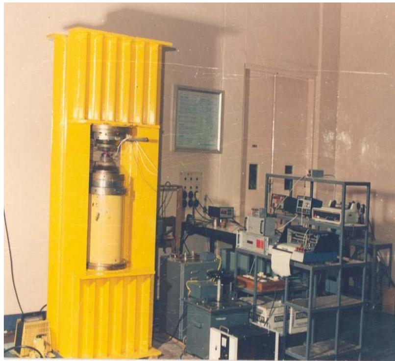
**Fig.2.1.** Photograph of the 500 T hydraulic press. The main components are hydraulic pump, digital pressure indicator, and high current transformer [6].
