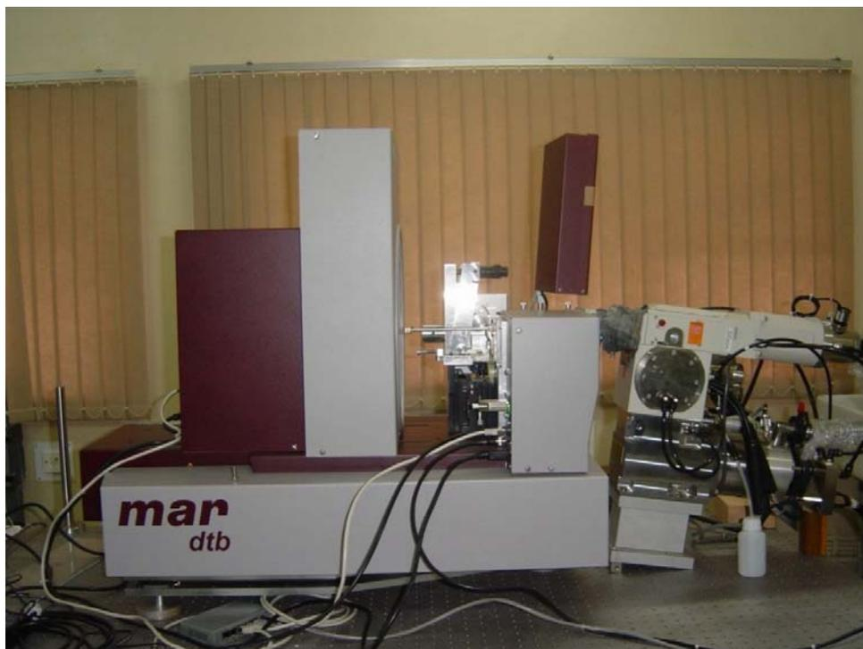
**Fig.2.8.** High Pressure Angle Dispersive X-ray Diffraction system used for the high pressure experiments at our laboratory.
