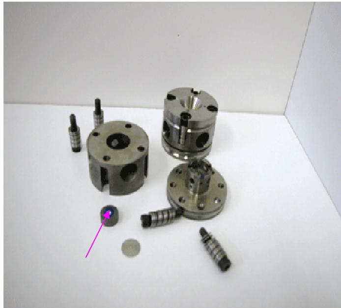
**Figure 3.1:** *Diamond Anvil Cell assembly. Arrow mark indicates the location of the diamond. The culet size is 300 micron.*
