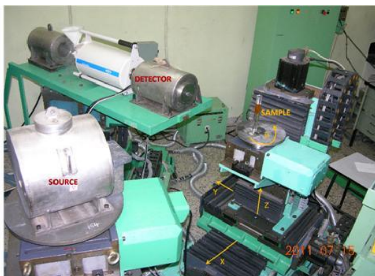
Figure 4.1 Experimental set-up with source, sample and detector labeled.
