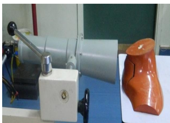
Fig.2.4 Thyroid Monitor with Thyroid phantom
