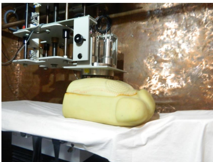
Fig.2.11 Counting geometry for liver measurement
