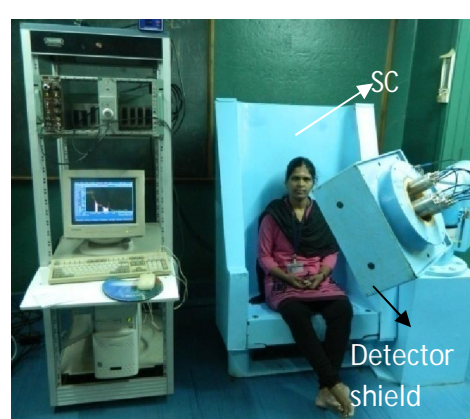
Fig.2.3 SC counter with a) Masonite phantom and b) subject
