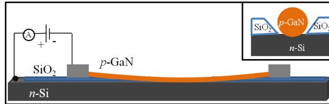
Fig. 6.9 A schematic cross-sectional side-view (along the NW) of a single NW  $p$ - $\text{GaN}/n$ - $\text{Si}$  heterojunction device in the forward bias configuration. Inset shows the cross-sectional (across the NW) front-view of the device.
