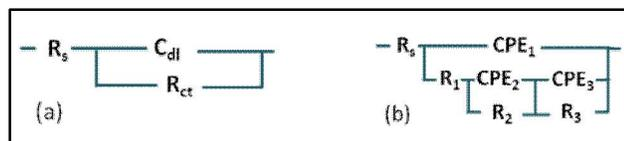
Figure 5.9: (a) Simple Randles circuit, and (b) modified electrical equivalent circuit for VGN3 electrode in aqueous medium
