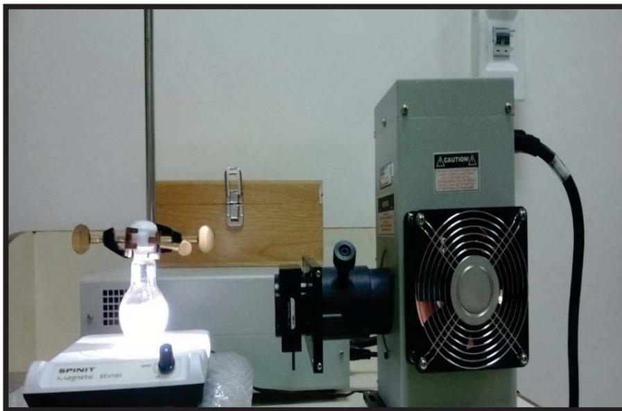
**Figure 2.12** Photocatalytic hydrogen generation test done under AM 1.5 illuminations (100 mW/cm<sup>2</sup>) for 10 mg of photocatalyst in 40 ml aqueous ethanol solution.
