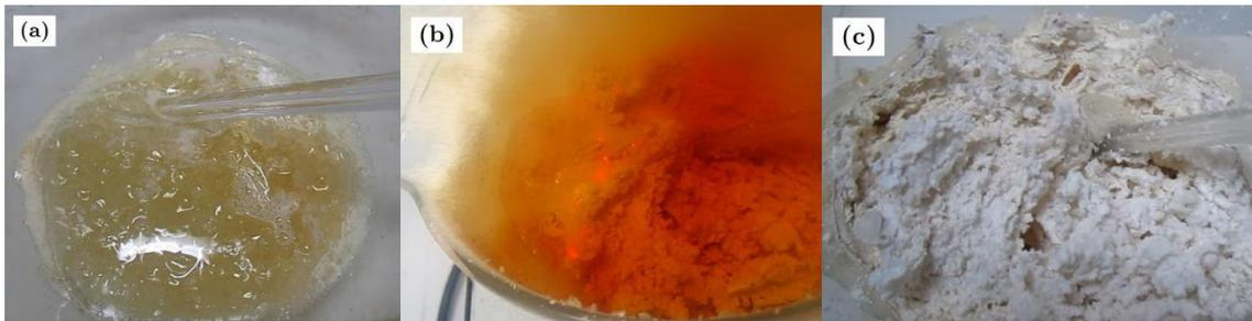
Figure 2.2 The photographs depicting the stages in the synthesis of thoria from the precursors thorium nitrate and citric acid, by citrate gel combustion method. (a) the gel before combustion, (b) combustion and (c) after combustion.
