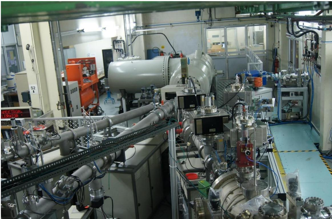
Figure 2.4 Photograph of 1.7 MV Tandetron accelerator and the beamlines.
