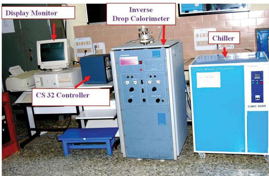
**Fig. 3.6.** The experimental setup for Inverse Drop calorimeter used in the present study
