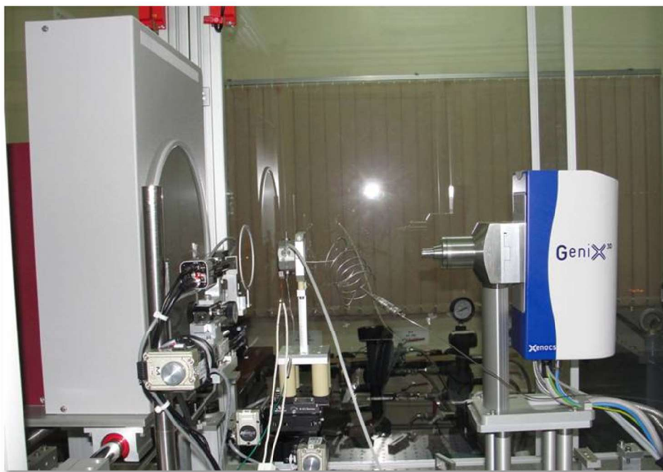
Figure 3.6: Novel set up of micro-focus XRD attached with membrane cell DAC
