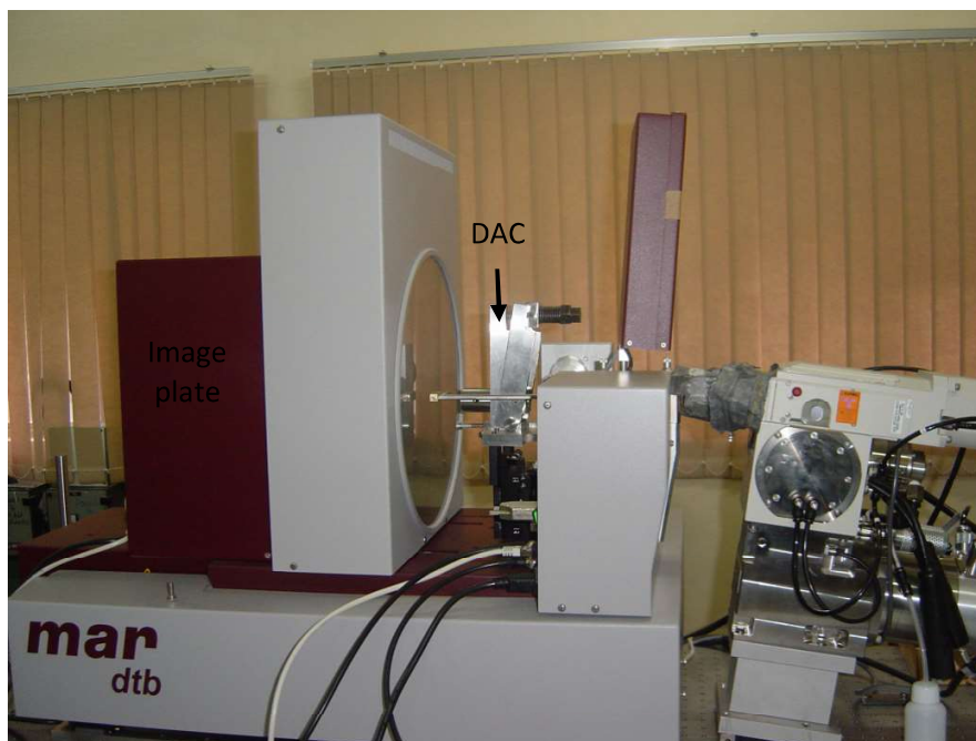
Figure 2.7: Rigaku ULTRAX18 (18 kW) rotating anode X-ray generator loaded with Mao-Bell type DAC
