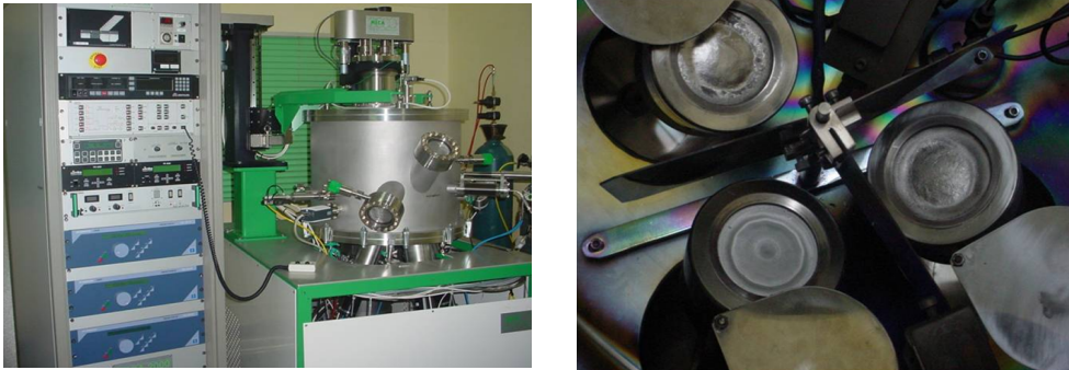
Figure 2.1 – Photograph of the sputtering unit (MECA 2000-France) and the arrangement of guns covered by targets.
