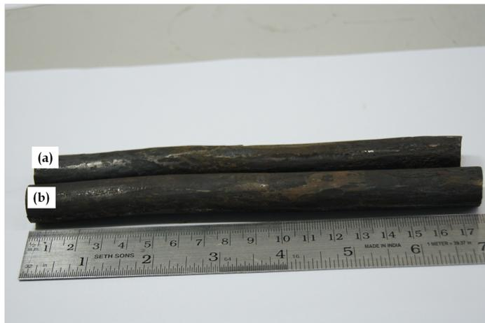
**Figure 4.1:** As prepared (a) Fe-14Cr-0.63Zr-4Al-0.3Y<sub>2</sub>O<sub>3</sub>(Al-ODS) and (b) Fe-14Cr-0.63Zr-0.3Y<sub>2</sub>O<sub>3</sub>(Zr-ODS) rods
