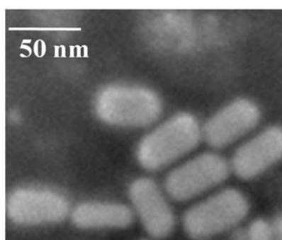
Figure 3.2 FESEM micrograph of Au NRs.
