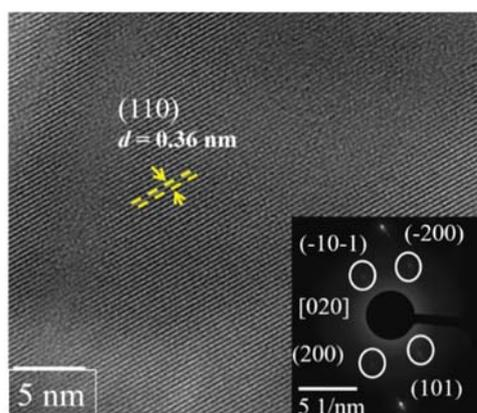
Figure 2.18 TEM images of SnO<sub>2</sub> micro-belt (inset) SAED pattern obtained along [020] zone axis.
