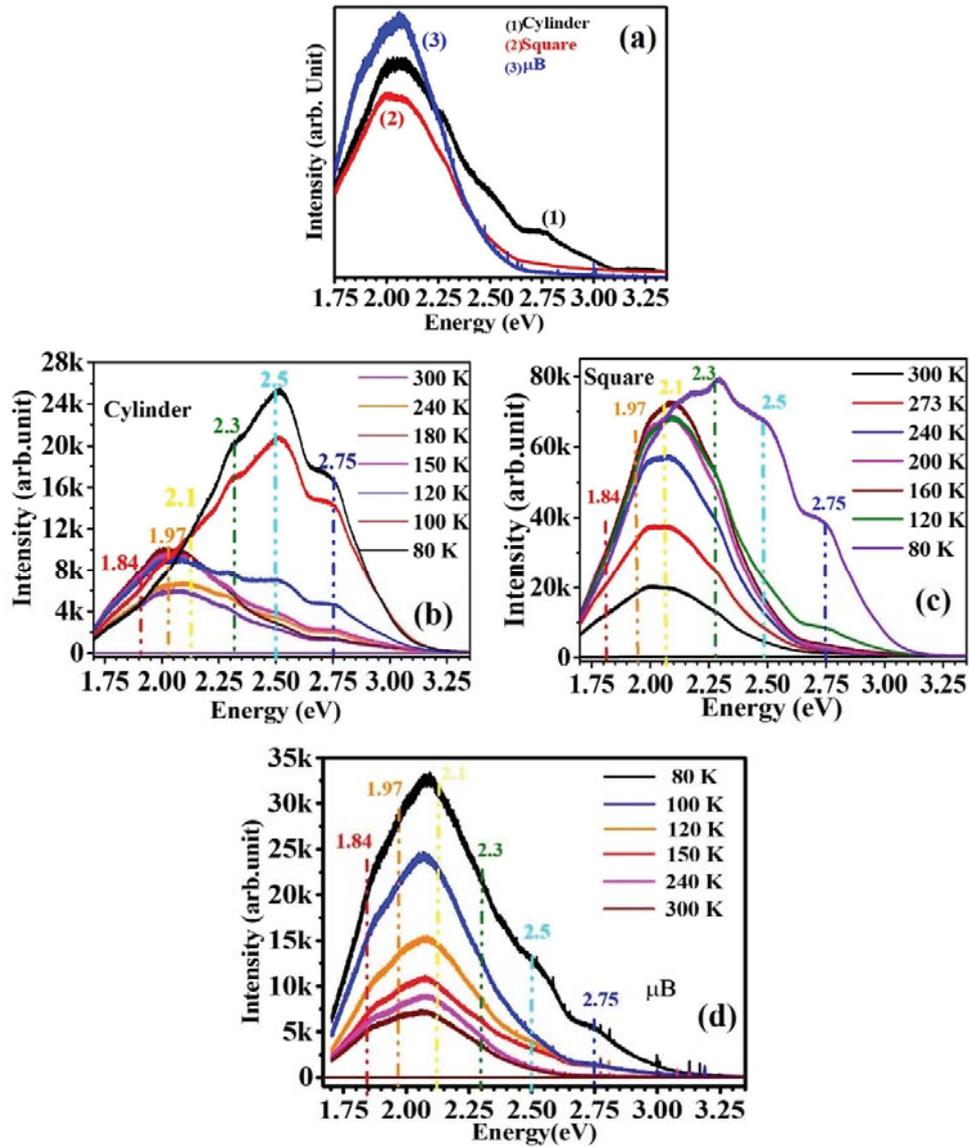
Figure 4.18 (a) PL spectra collected from all 1-D NSs, temperature-dependent PL studies of (b) cylindrical, (c) square-shaped nanowire, and (d)  $\mu$ B.
