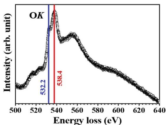
Figure 5.2 EELS of SnO<sub>2</sub> QDs in the carbon matrix.
