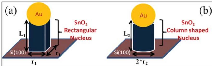
Figure 2.15 Schematic of the VLS growth mechanism for (a) Square and (b) Cylinder shaped NWs
