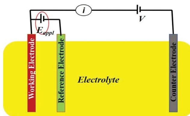
Figure 5.4 Three electrode system for electrochemical measurement.
