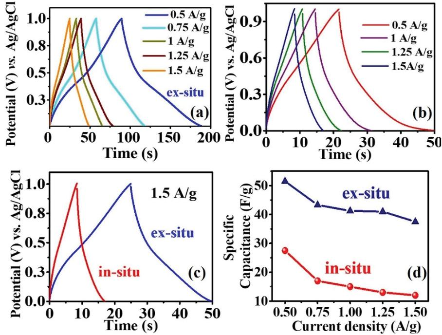
Figure 5.12 Charging discharging of GO-SnO<sub>2</sub> (a) ex-situ (b) in-situ at different current densities; (c) CD of the in-situ and the ex-situ samples at a current density of 1.5 A g<sup>-1</sup> (d) specific capacitance vs. current density.
