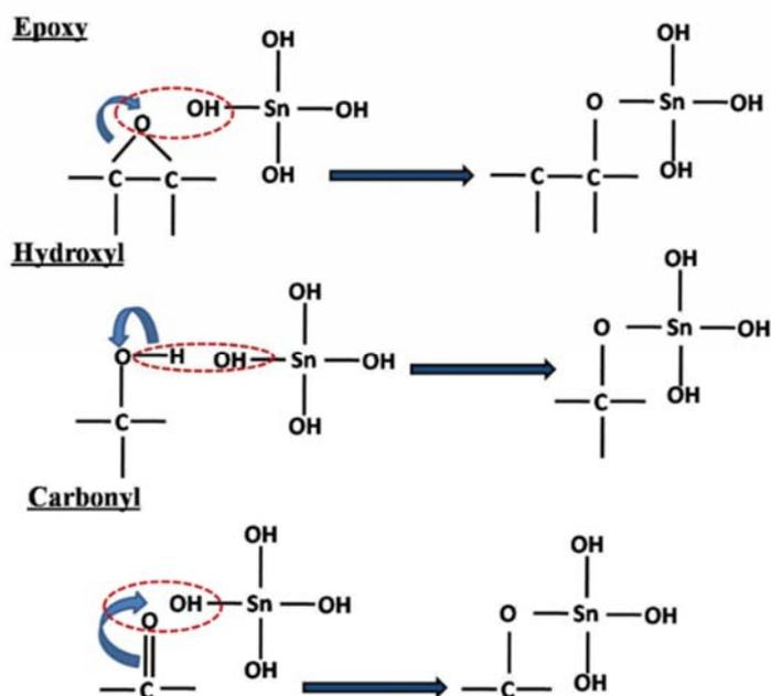
Figure 2.26 Schematic representation of possible reaction pathways for functional groups of GO during the formation of nucleation for SnO<sub>2</sub> NPs.
