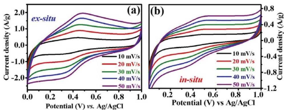
Figure 5.10 Cyclic voltammetry study of GO-SnO<sub>2</sub> (a) ex-situ and (b) in-situ at various scan rates.
