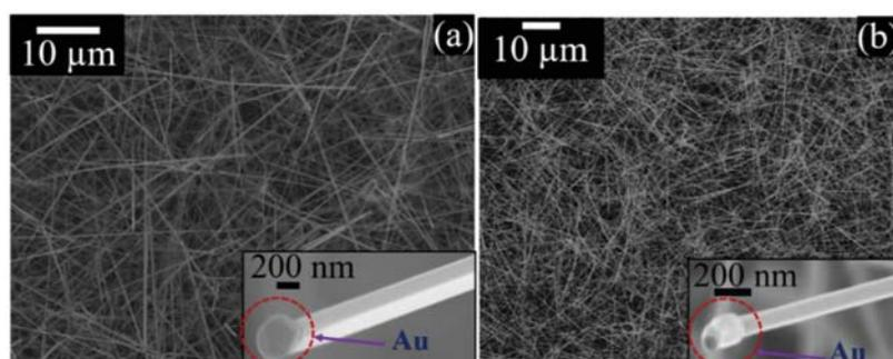
Figure 2.12 FESEM images of NWs grown at (a) 950 °C and (b) 1000 °C. Insets are high-resolution FESEM for NWs with Au droplet.
