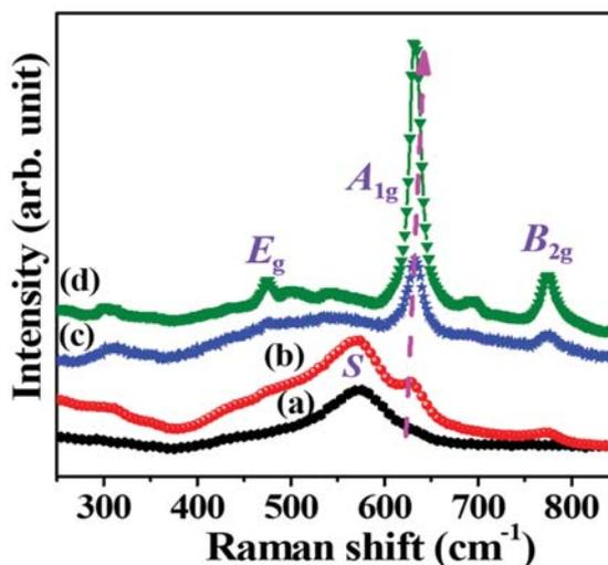
Figure 2.7 Raman spectra of SnO<sub>2</sub> NPs (a) A (100 °C), (b) B (200 °C), (c) C (500 °C) and (d) D (800 °C).
