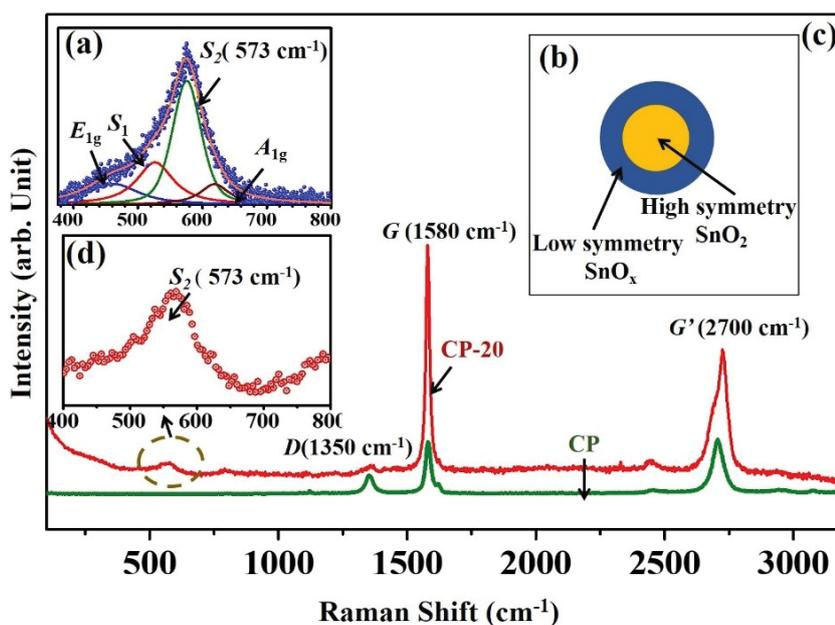
Figure 5.3 (a) Raman spectrum of SnO<sub>2</sub> QDs with Lorentzian fitting (b) schematic view of SnO<sub>2</sub> NPs with the depiction of non-stoichiometric layer (c) Raman spectra of CP and CP-20 (d) Zoomed version of the defect-related peak in SnO<sub>2</sub> from CP-20.
