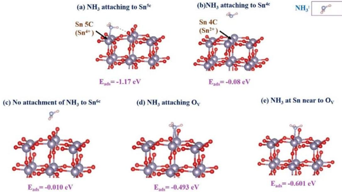
Figure 4.14 Scheme of the adsorption of  $\text{NH}_3$  at different sites of  $\text{SnO}_2$  (110) surfaces.
