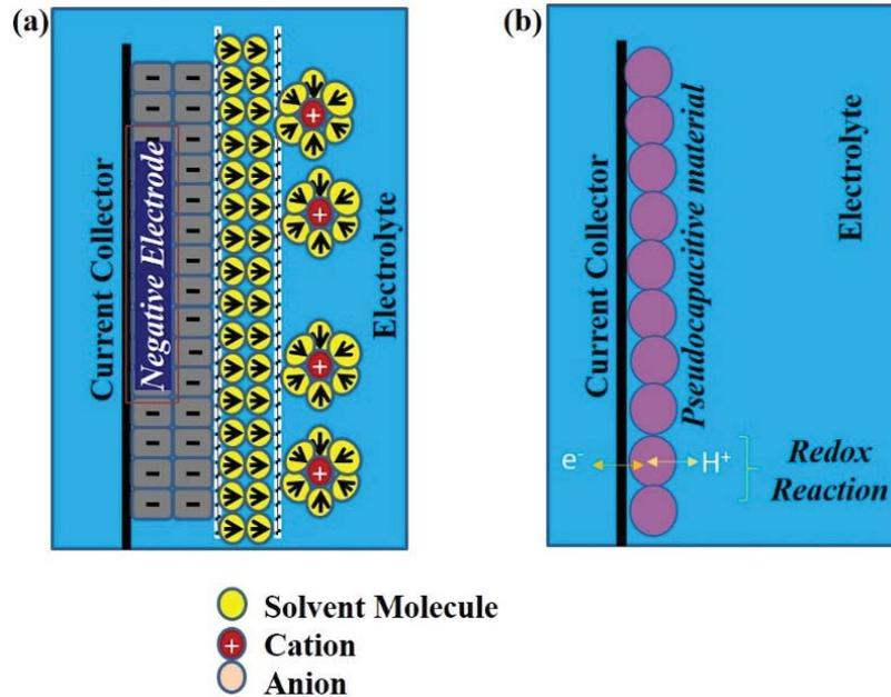
Figure 1.6 Charge storage mechanism in (a) electrical double-layer capacitance and (b) pseudocapacitance.
