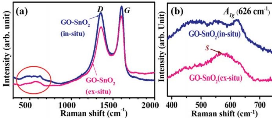
Figure 2.23 Raman spectra of (a) GO-SnO<sub>2</sub> composite and (b) SnO<sub>2</sub> portion in the composite
