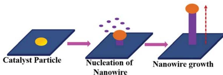
Figure 2.11 Schematic growth of vapor-liquid-solid growth.
