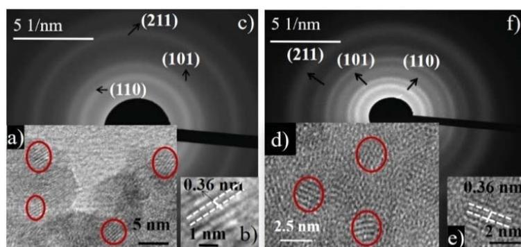
Figure 5.1 (a) TEM images, (b) lattice spacing, and (c) SAED patterns of SnO<sub>2</sub> QDs. (d) TEM image (b) lattice spacing and (f) SAED patterns of SnO<sub>2</sub> QDs in carbon paper matrix.
