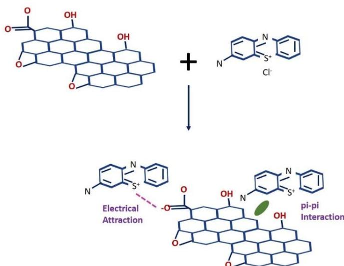
Figure 5.20 Schematic illustration for the adsorption mechanism of MB on the GO surface.
