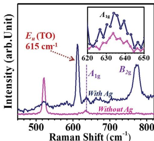
Figure 3.8 Raman spectra of sample D (800 °C) with and without Ag nanonets.
