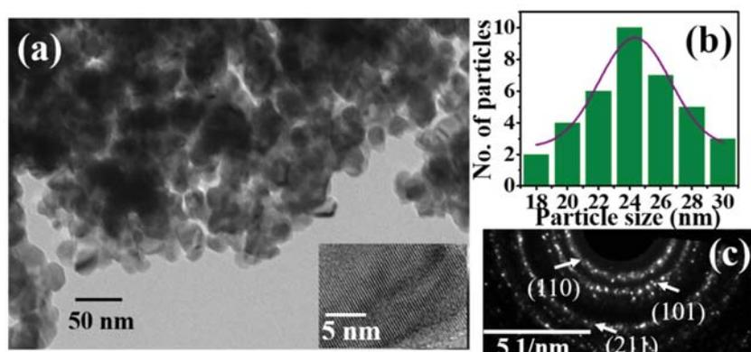
Figure 2.6 (a) HRTEM image (inset) interplanar spacing, (b) Particle size distribution with Gaussian fitting, and (c) SAED pattern of sample D (800 °C)
