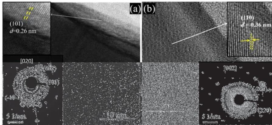
Figure 2.13 TEM image of (a) square shape NWs grown at 950 °C with [top inset (101) plane of rutile SnO<sub>2</sub> and bottom inset SAED pattern obtained along the [020] zone axis and (b) cylindrical shape NWs grown at 1000 °C with [top inset (110) plane of rutile SnO<sub>2</sub> and bottom inset SAED pattern obtained along the [002] zone axis.
