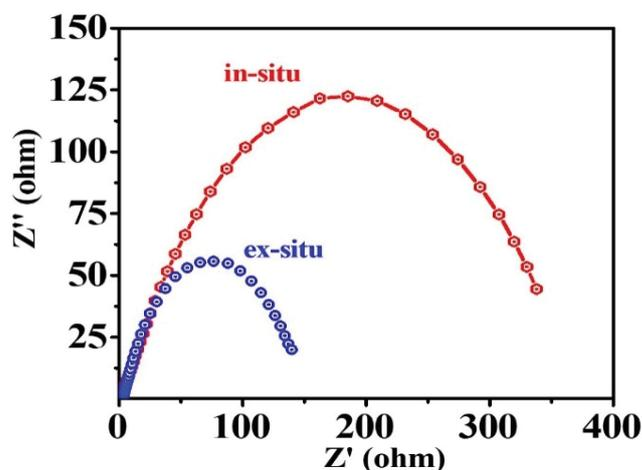
Figure 5.14 Impedance spectra for GO-SnO<sub>2</sub> composite.
