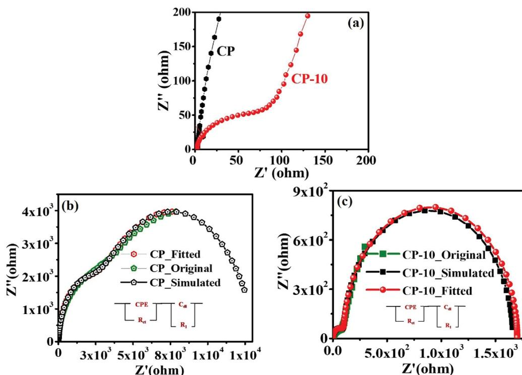
Figure 5.8 (a) Nyquist plot for CP and CP-10, Fitted Nyquist plots for (b) CP, and (c) C-10 with equivalent circuits.
