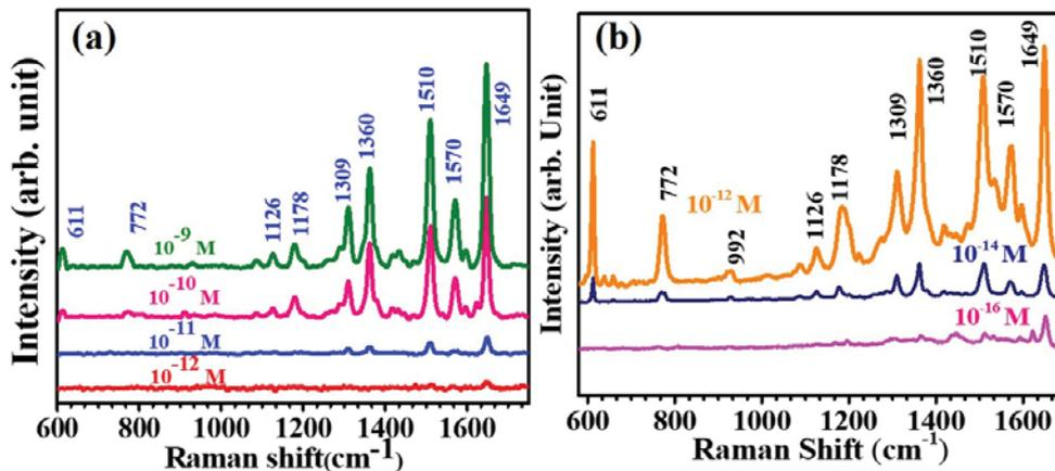
Figure 3.5 SERS collected from the different concentrations of R6G in the presence of (a) Au NRs and (b) Ag nanonets.
