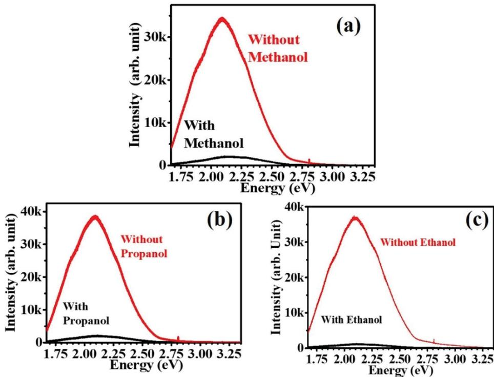
Figure 4.16 Displaying changes observed in PL signals after exposing to (a) methanol, (b) propanol, and (c) ethanol.
