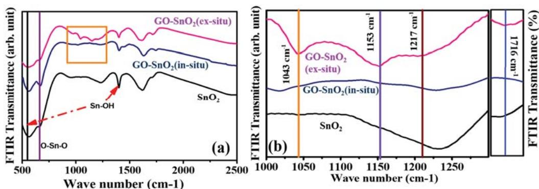
Figure 2.25 (a) FTIR spectra of SnO<sub>2</sub> and GO-SnO<sub>2</sub> composites (b) highlighting presence/absence of functional groups in the ex-situ and the in-situ GO-SnO<sub>2</sub> composites.
