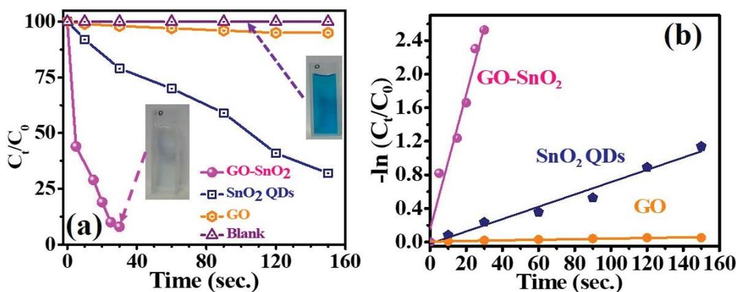
Figure 5.18 (a)  $C_t/C_0$  vs. irradiation time for photo-degradation of MB while the inset shows color of MB before (top) and after (bottom) degradation and (b) photocatalytic reaction kinetics.
