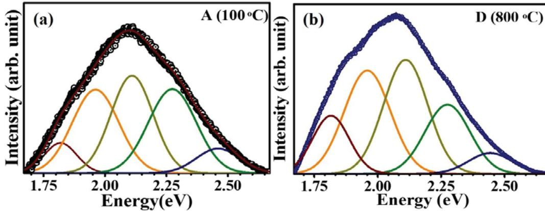
Figure 4.4 Convolved PL spectra of (a) A (100 °C) and (b) D (800 °C).
