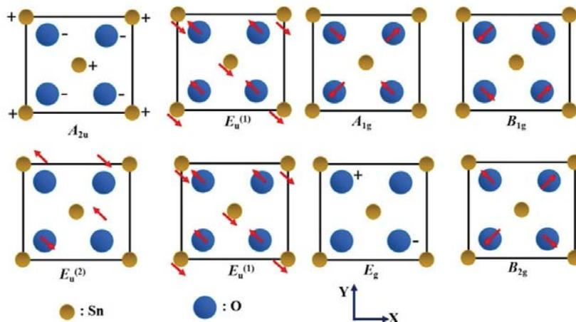
Figure 1.4 2-D representation of optical active vibrational modes along the *c*-axis of the unit cell and the movement of atoms in-plane is indicated by arrows, while (+) and (-) for movement along the *c*-axis.
