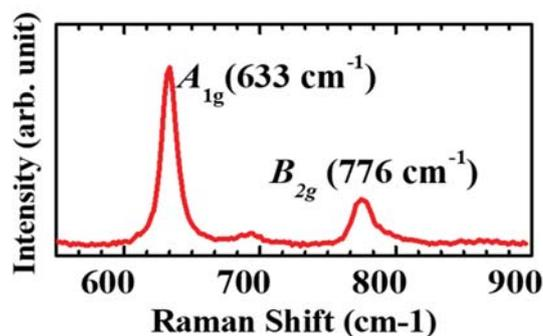
Figure 2.19 Raman spectra of a single SnO<sub>2</sub> micro-belt.
