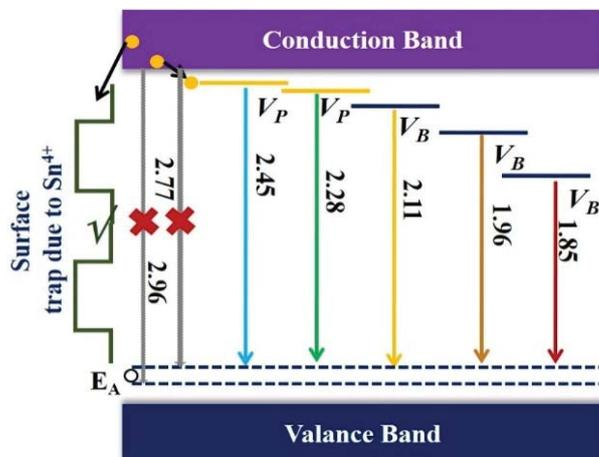
Figure 4.9 Band diagram for  $\text{SnO}_2$  NPs showing different PL transition levels.
