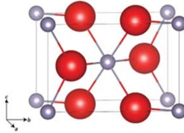
Figure 1.1  $\text{SnO}_2$  unit cell with Sn (IV) state in grey and O in solid.
