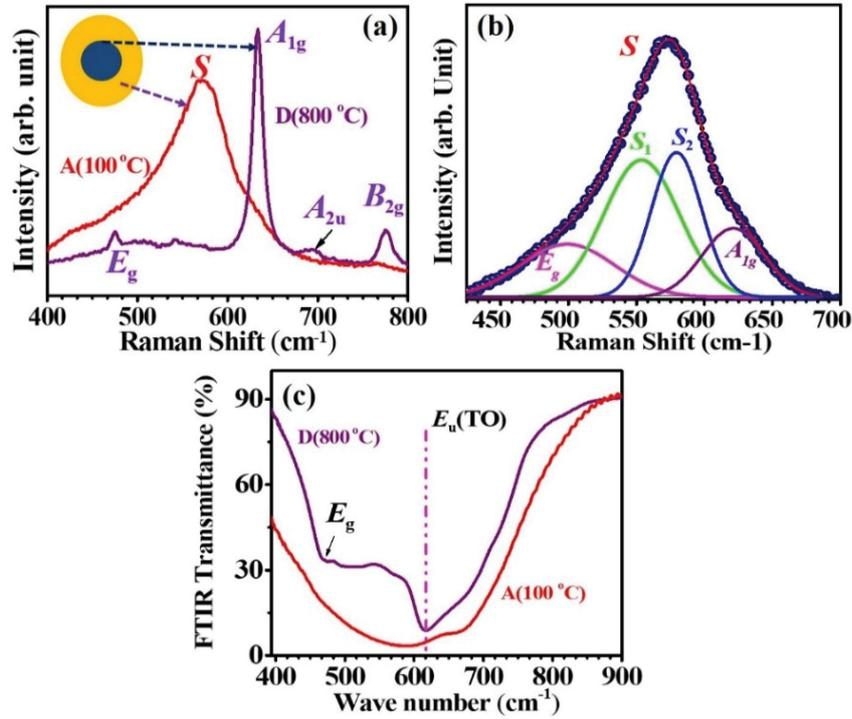
Figure 3.7 (a) Raman spectra of SnO<sub>2</sub> NPs, (b) deconvoluted Raman spectrum of A (100 °C) (c) FTIR spectra of SnO<sub>2</sub> NPs.
