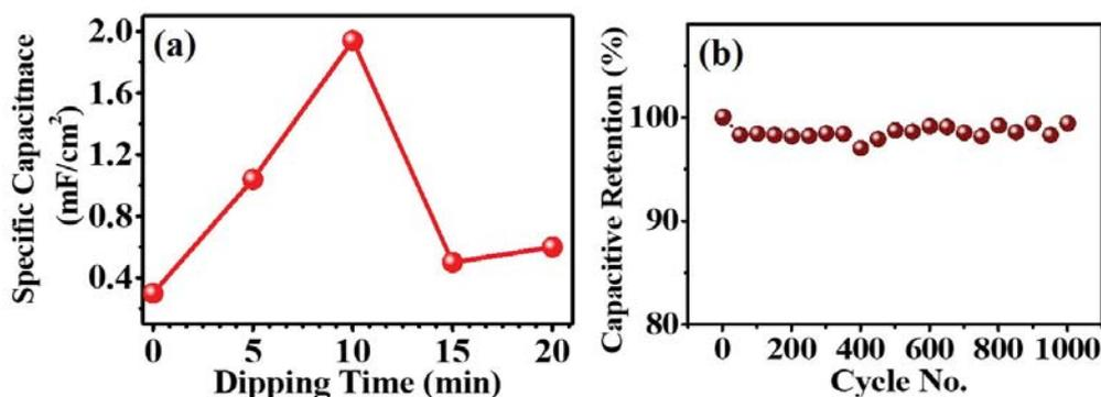
Figure 5.7 (a) Specific capacitance with respect to dipping time calculated from charging-discharging plot (b) Cyclic stability of CP-10.
