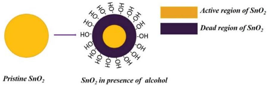
Figure 4.17 Scheme of the active and dead region of  $\text{SnO}_2$  NP as created before and after exposure to alcohol.
