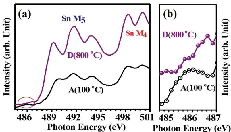
Figure 4.7 (a) Sn  $M_{4,5}$  edge XANES spectra of SnO<sub>2</sub> NPs (b) Zoom of the encircled part of Fig (a).
