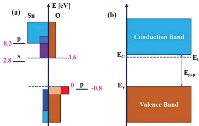
Figure 1.3 Schematic representation of the density of states for valence band and conduction band (b) simplified band diagram of SnO<sub>2</sub> with a donor state ( $E_D$ ) close to the conduction band.
