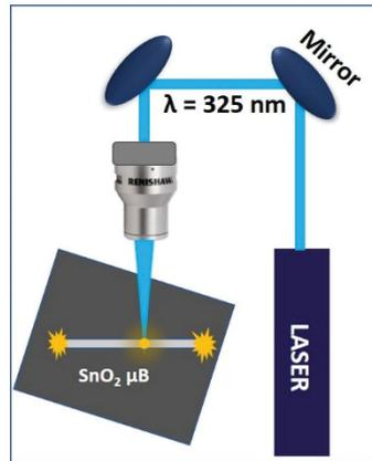
Figure 4.19 Schematic view for the waveguide study of 1-D  $\text{SnO}_2$  NSs.
