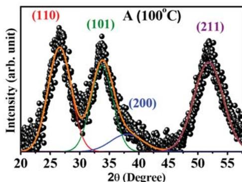
Figure 2.2 Gaussian fitting of XRD patterns of A (100 °C)
