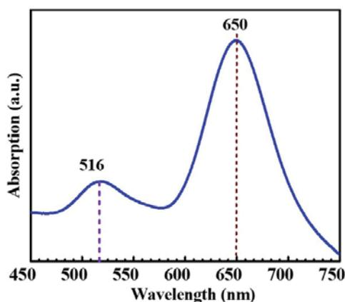
Figure 3.1 UV-Visible spectrum of Au NRs with LSPR at 650 nm.
