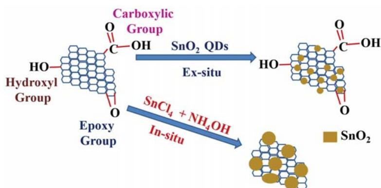
Figure 2.27 Schematic representation of decoration of SnO<sub>2</sub> NPs on the surface of GO sheet by both ex-situ and in-situ process of synthesis.
