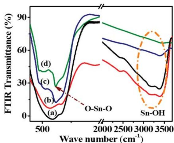
Figure 2.8 FTIR spectra of (a) A (100 °C), (b) B (200 °C), (c) C (500 °C) and (d) D (800 °C)
