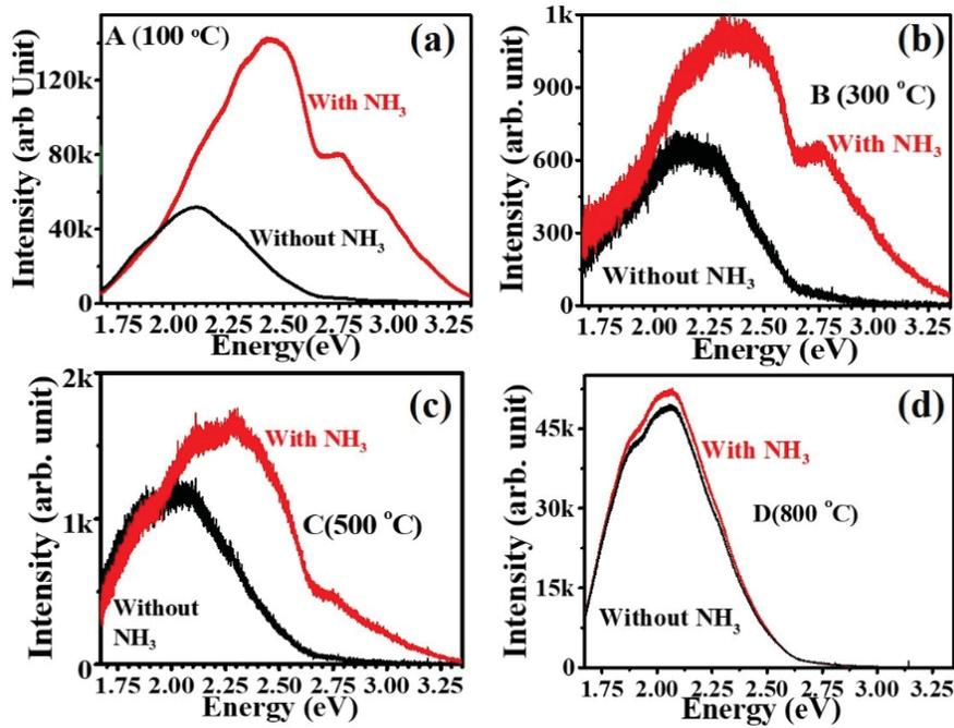
Figure 4.3 PL collected in the absence and presence of  $NH_3$  for (a) A (100 °C), (b) B (300 °C), (c) C (500 °C), and (d) D (800 °C) samples.
