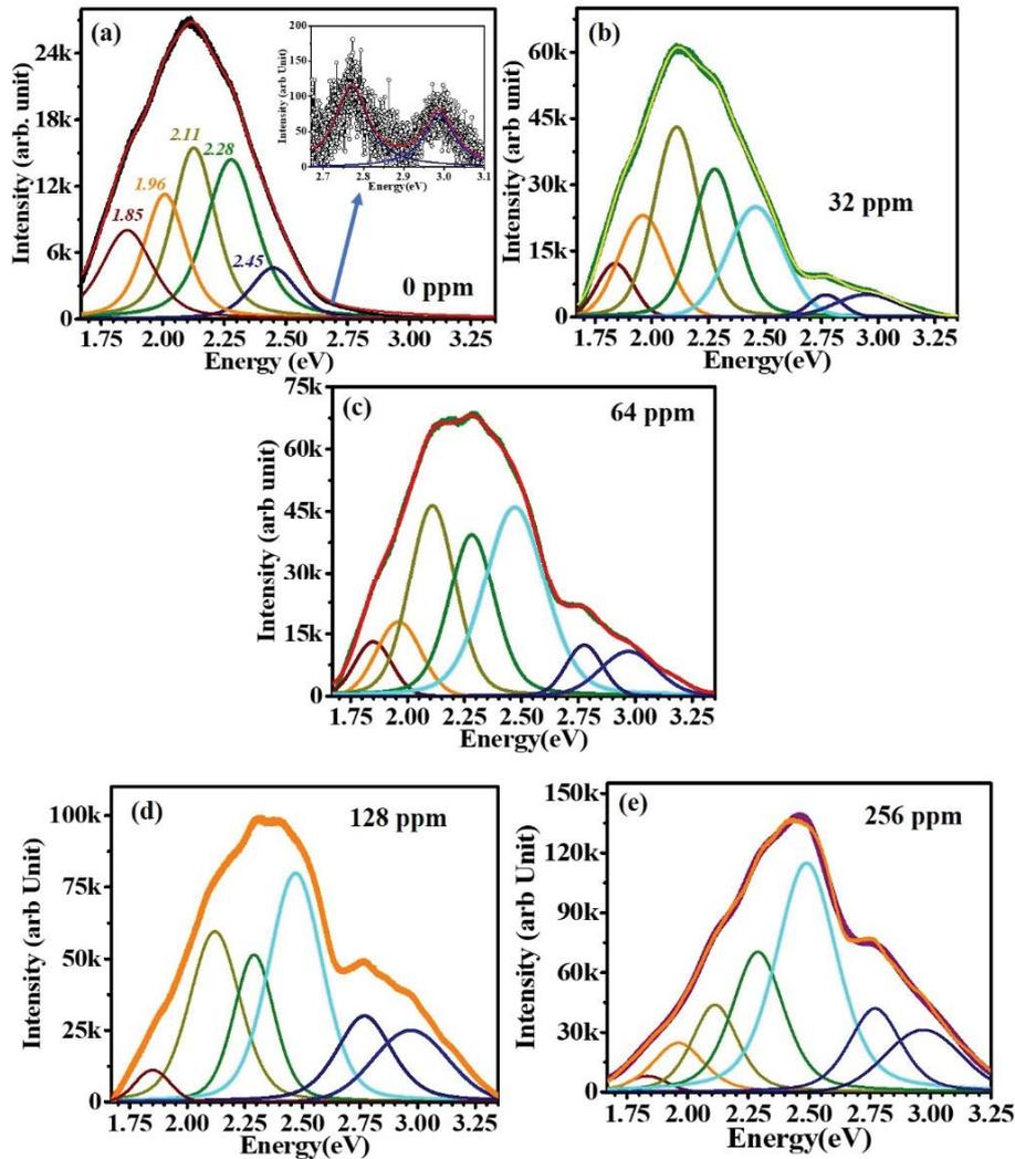
Figure 4.11 Convolved PL spectra of the  $\text{SnO}_2$  QDs exposed to (a)0, (b)32, (c) 64, (d)128 and (e)256 ppm of  $\text{NH}_3$ .
