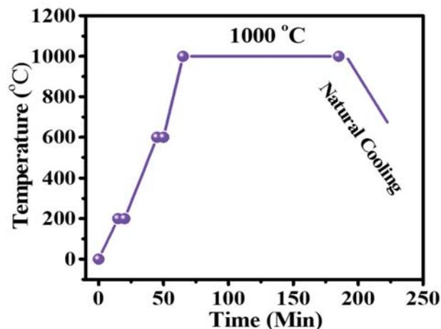
Figure 2.16 Temperature profile maintained during the growth process
