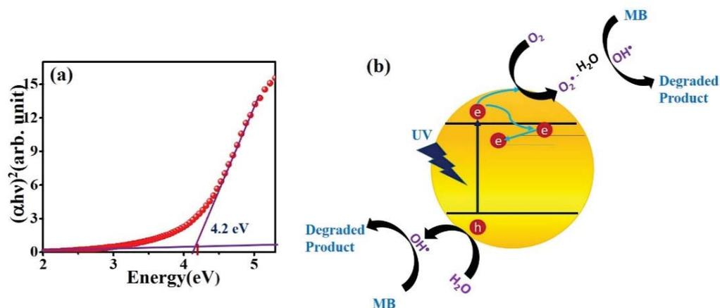
Figure 5.16 (a) UV-Vis spectrum of SnO<sub>2</sub> QDs (b) MB degradation in the presence of SnO<sub>2</sub> QDs with UV illumination.
