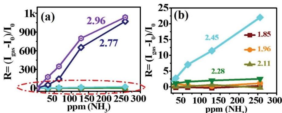
Figure 4.12 (a) Sensor responses of QDs for all the peak positions, (b) zoomed version of the encircled part for peaks,  $V_P$  and  $V_B$ .
