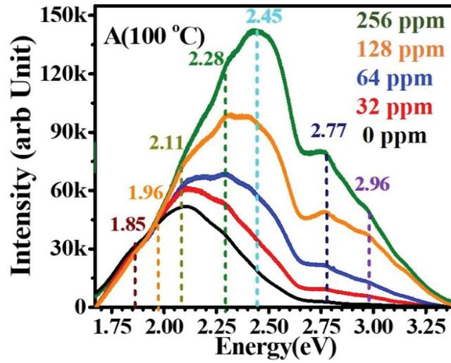
Figure 4.10 PL spectra collected in the presence of different concentrations of  $NH_3$ .
