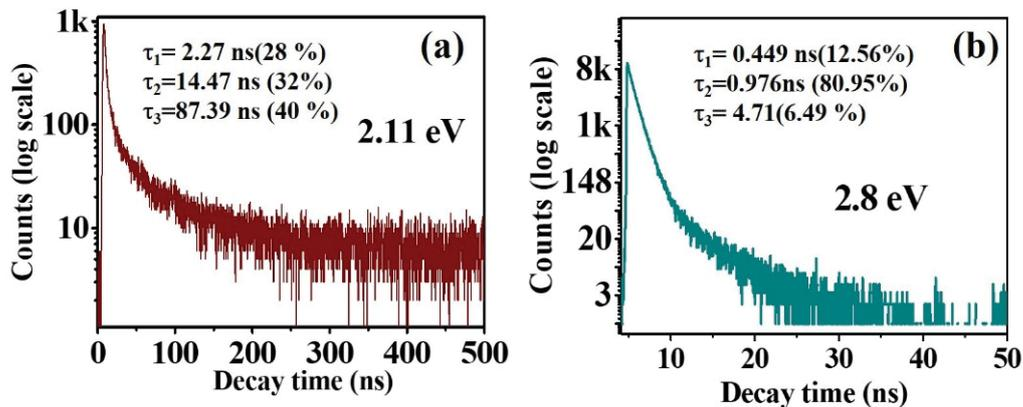
Figure 4.8 Lifetime measurements of SnO<sub>2</sub> QDs for the emissions at (a) 2.27 and (b) 2.8 eV.
