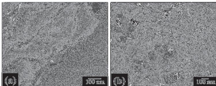
Figure 2.21 FESEM images of (a) GO-SnO<sub>2</sub> (in-situ) and (b) GO-SnO<sub>2</sub> (ex-situ)
