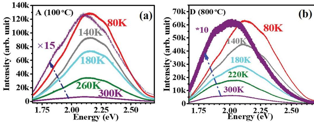
Figure 4.5 Temperature dependent PL spectra of (a) A (100 °C) and (b) D (800 °C) samples.
