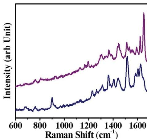
Figure 3.6 Variation of the Raman intensity with time indicating the blinking effect of R6G molecule.
