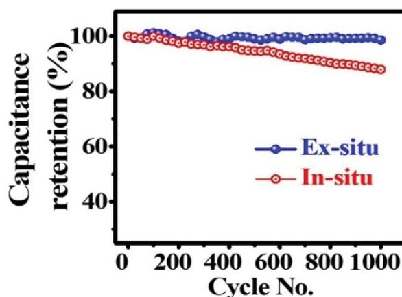
Figure 5.13 Retention of the capacitance of GO-SnO<sub>2</sub> composites.
