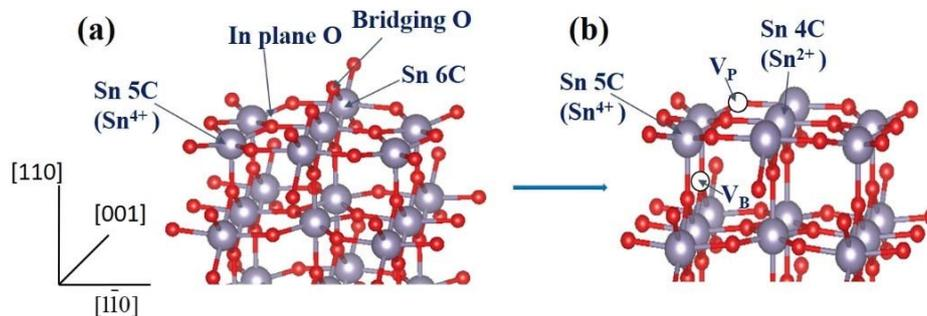
Figure 1.2 Side view of the SnO<sub>2</sub> (110) stoichiometric surfaces. The large (small) spheres represent tin (oxygen) atoms. Oxygen atoms are labelled according to the convention discussed in the text.
