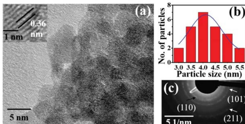
Figure 2.4 (a) HRTEM image of the sample B (300 °C) with interplanar spacing as inset, (b) Particle size distribution with Gaussian fitting and (c) SAED patterns
