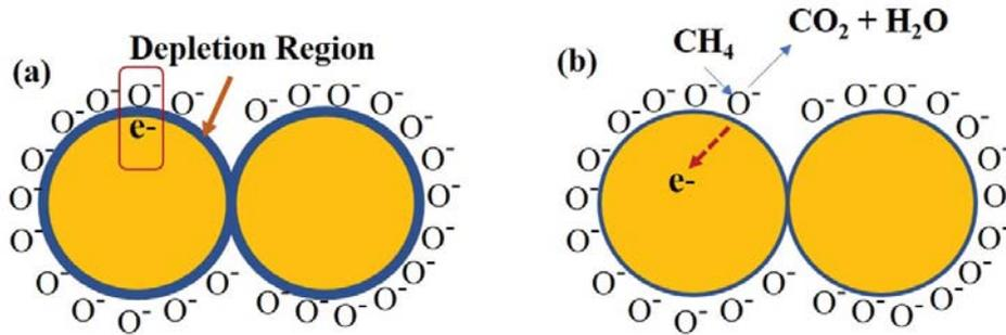
Figure 1.5 (a) Highlight of depletion region formation (b) after effect of an interaction with CH<sub>4</sub> with SnO<sub>2</sub>.
