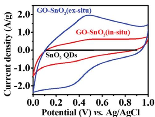
Figure 5.9 CV of in-situ, ex-situ, and as-prepared SnO<sub>2</sub> QDs at a scan rate of 50 mV/s.
