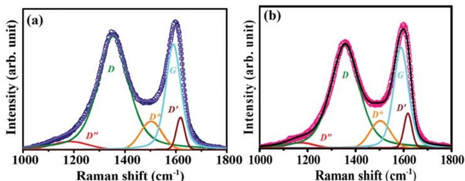
Figure 2.24 Deconvoluted Raman spectra of (a) GO-SnO<sub>2</sub> (in-situ) and (b) GO-SnO<sub>2</sub> (ex-situ)
