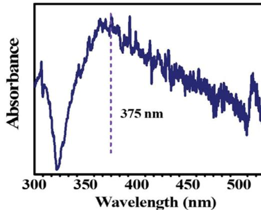
Figure 3.3 UV-Vis spectrum of Ag nanonets on Si substrate.
