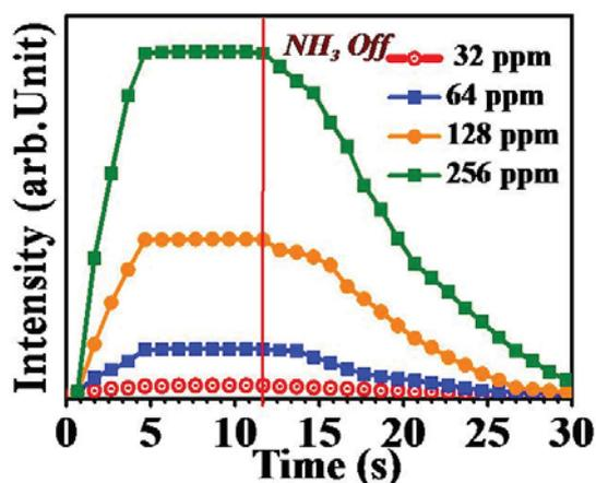
Figure 4.15 Sensor response and recovery time with reference to the intensity of 2.77 eV peak of SnO<sub>2</sub> QDs. The vertical line indicates the starting point of the recovery of a PL sensor with N<sub>2</sub> purge.
