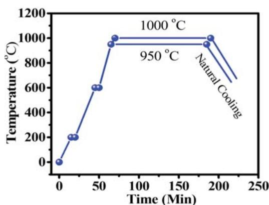
Figure 2.10 Temperature profile maintained during the growth process
