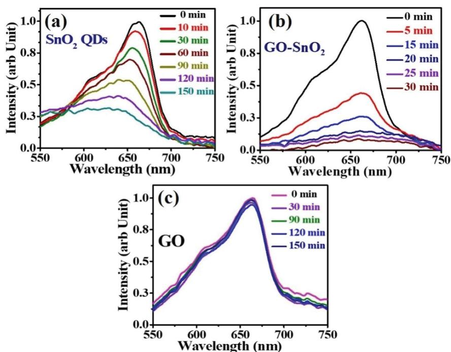
Figure 5.17 Time-dependent UV-Vis absorption spectra of MB in the presence of (a) SnO<sub>2</sub> QDs (b) GO-SnO<sub>2</sub> and (c) GO.
