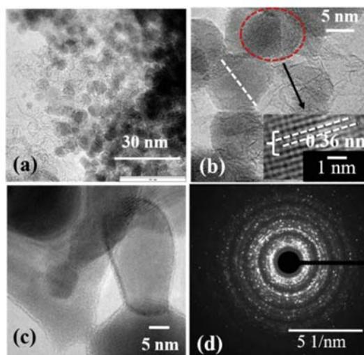
Figure 2.22 (a), (b), (c) Irregular shaped TEM images of SnO<sub>2</sub> nanoparticles in GO matrix. (d) SAED patterns of SnO<sub>2</sub> collected from SnO<sub>2</sub> NPs.
