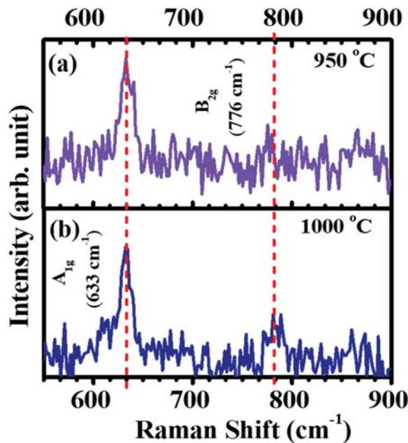
Figure 2.14 Raman spectra collected from (a) square shape and (b) cylindrical shape NWs.
