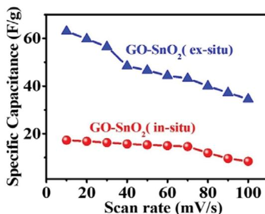
Figure 5.11 The specific capacitance of GO-SnO<sub>2</sub> composites at various scan rates.
