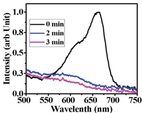
Figure 5.15 Time-dependent UV-Vis absorption spectra of MB with SnO<sub>2</sub> QDs under the UV irradiation.
