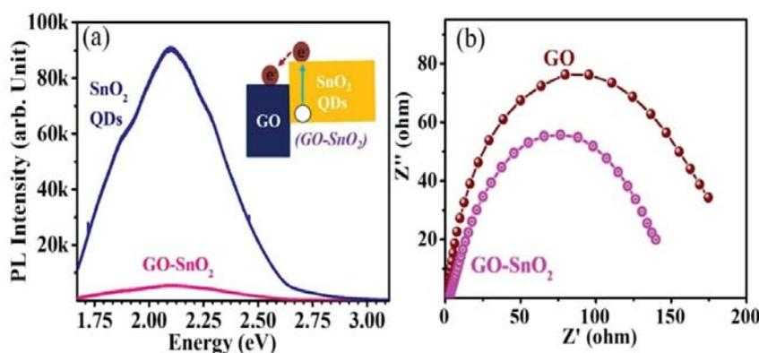
Figure 5.21 (a) PL spectra of SnO<sub>2</sub> QDs and GO-SnO<sub>2</sub> with an inset to show an electron transfer from QDs to GO (b) EIS spectra of GO and GO-SnO<sub>2</sub> composite.
