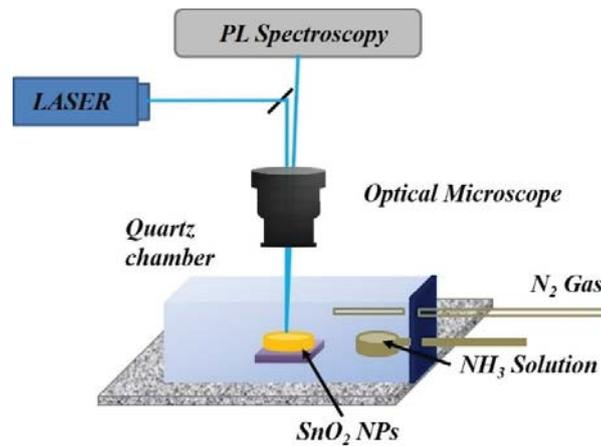
Figure 4.2 Schematic view of the set-up used for PL sensor study with different analytes.
