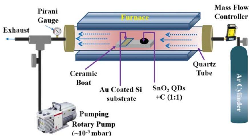
Figure 2.9 Schematic representation of the CVD system used for the growth of various forms of SnO<sub>2</sub> nanostructures.
