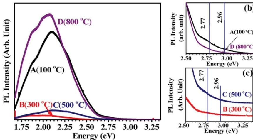
Figure 4.1 PL of SnO<sub>2</sub> NPs at (a) RT and existence of peaks at 2.77 and 2.96 eV for samples (b) A&D and (c) B&C
