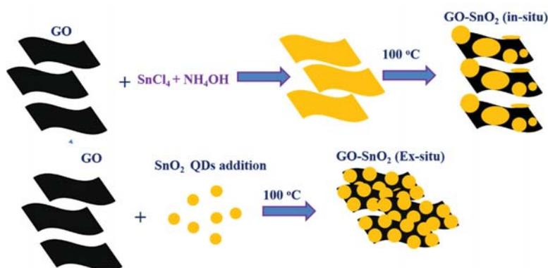
Figure 2.20 Schematic view of in-situ and ex-situ synthesized GO-SnO<sub>2</sub>.
