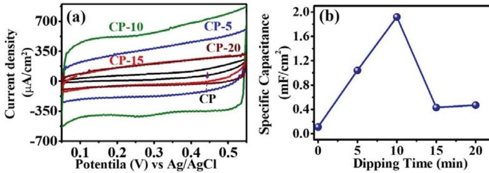
Figure 5.5 (a) CV and (b) specific capacitance for varied dipping time for all the electrodes.
