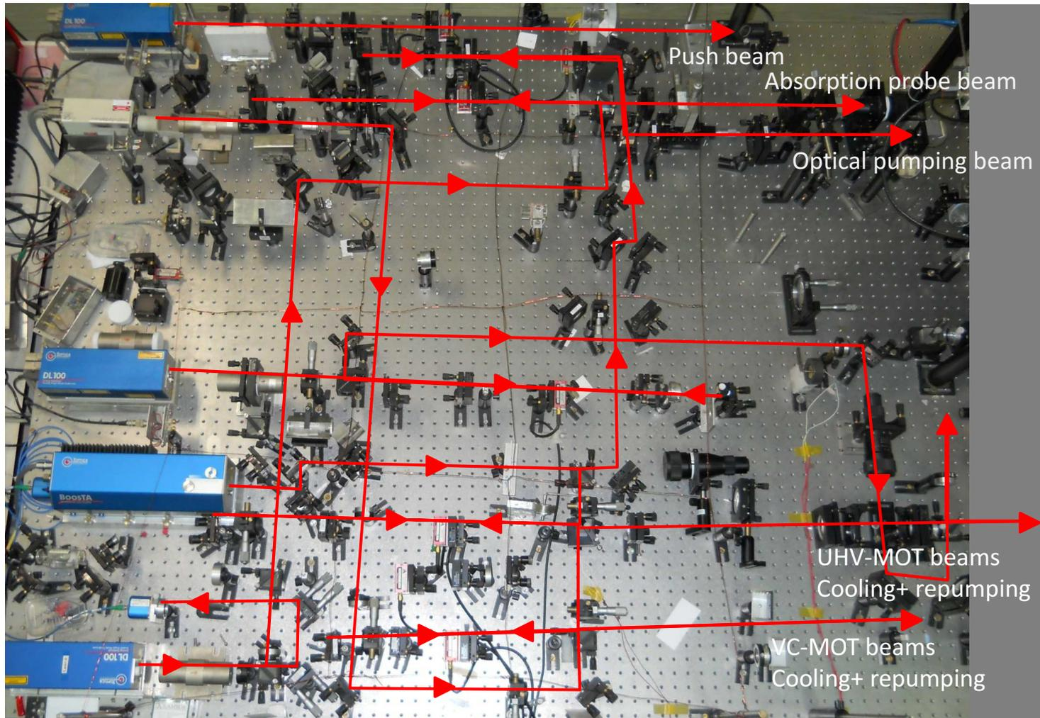
Figure 2.7: A photograph of the table. The lines shows the path of the various generated optical beams. The lines with double arrows represents the AOMs in double-pass configuration. The Splitting of VC-MOT beams and UHV-MOT beams are not shown here. Refer to the text for more details.
