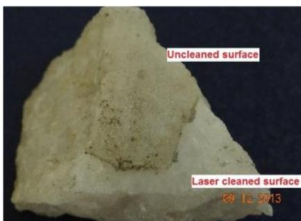
**Fig. 7.5.** Surface of the marble sample shows a clear difference between unclean and laser cleaned surface. After laser cleaning, the substrate colour becomes similar to the native substrate material.
