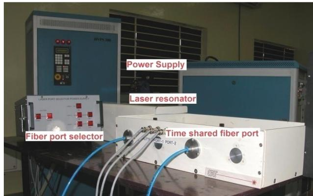
**Fig. 2.11.** A view of 250 W average power laser system with two time shared fiber optic port for beam delivery.
