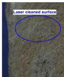
**Fig.7.8.** Surface of the berea gray sand stone sample shows a slight colour difference between the laser cleaned surface and native substrate surface.
