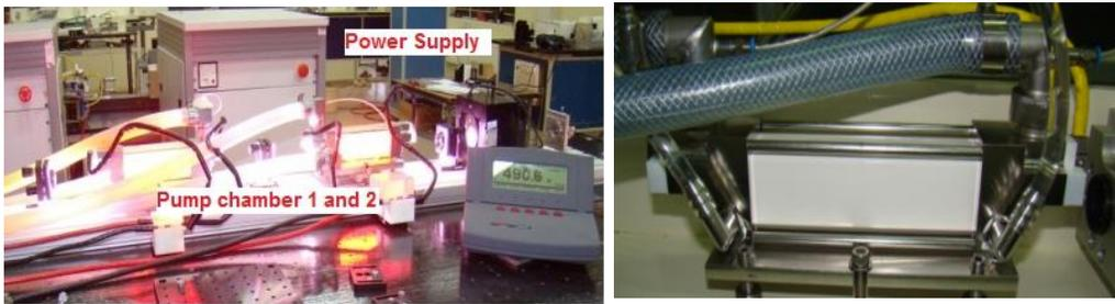
**Fig. 2.14.** A view of 500 W average power laser system and experimental set-up (left) and ceramic reflector (right).
