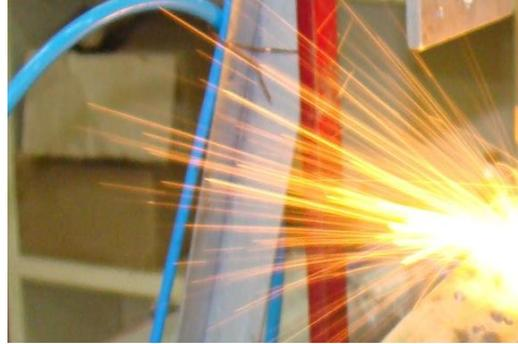
**Fig. 6.23.** A view of debris ejection during pulsed Nd:YAG laser cutting with 1:1 imaging nozzle.
