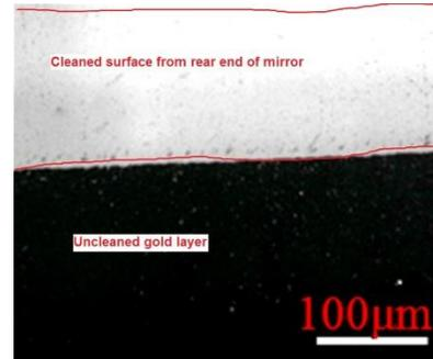
**Fig.7.20 (b).** *Microscope image of the cleaned surface, when it was cleaned from the rear surface. Some gold particles remain on surface (upper part) and lower part shows gold-coated uncleaned surface.*
