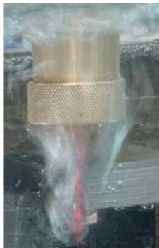
**Fig. 6.6.** A view of local dry cavity in underwater environment.
