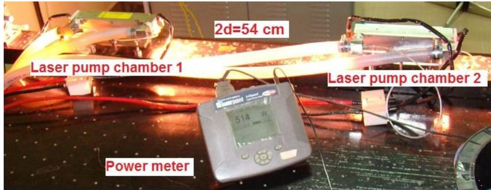
**Fig. 3.7.** A table top view of dual rod lamp pumped ceramic Nd:YAG resonator.
