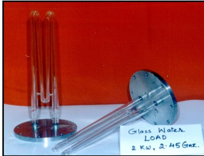
*Figure 4.40 : A photograph of the glass-water load.*
