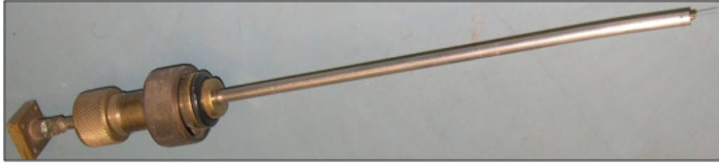
*Figure 7.5 : A photograph of indigenously developed Langmuir probe.*
