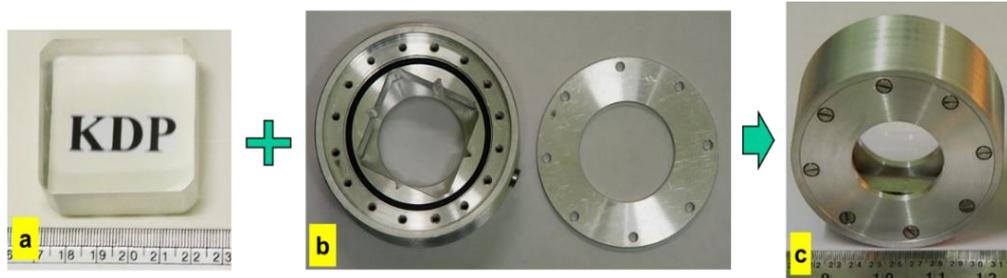
Fig. 3.44 (a) SHG element of size  $50 \times 50 \times 25 \text{ mm}^3$  prepared from a flat top KDP crystal, (b) a housing designed for the SHG element, and (c) complete KDP type-II SHG cell with antireflection windows and index matching fluid.
