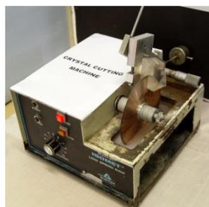
*Fig. 3.20 Slicing process of type-I SHG oriented KDP parallel to its base using Buehler make low speed saw.*
