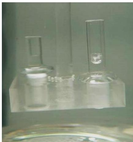
*Fig. 3.12 Seed holders of length 15 and 20 mm showing remaining KDP seed part in the longer tube after 47.5 hours of overheating.*
