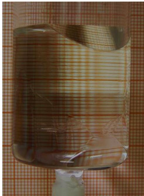
*Fig. 4.28 Unidirectional KDP crystal grown along (100) face by solute feeding technique.*
