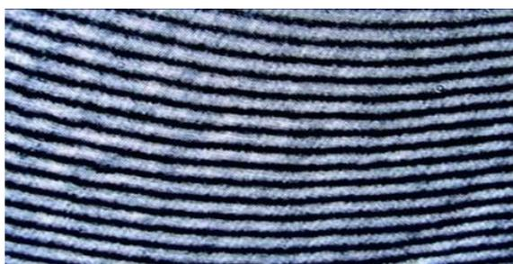
*Fig. 5.13 Mach-Zehnder interferogram of the (100) plate of the LAP crystal.*
