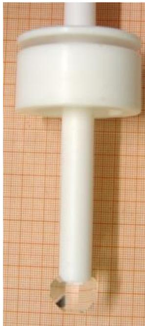
*Fig. 5.24 Photograph of the as-grown LAP crystal at the mount after the experiment.*
