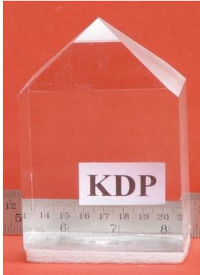
*Fig. 3.13 KDP crystal grown using seed protection technique.*
