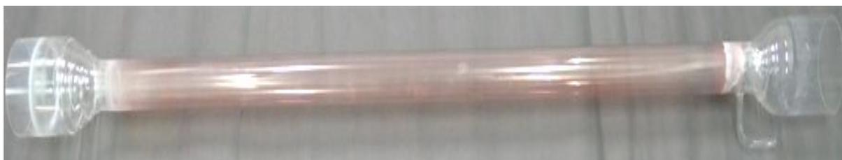
*Fig. 2.2 In-house developed fused silica discharge tube for Cu-HBrL*
