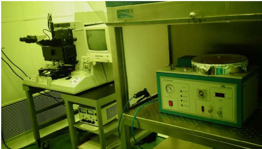
Figure 3.2 Actual photograph of the mask aligner and spin coating system
