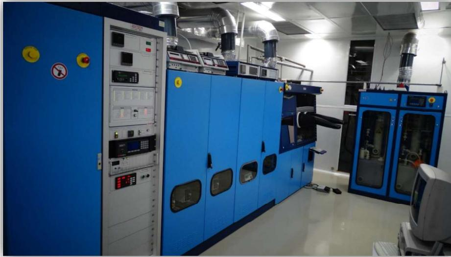
Figure 3.1 Photograph of MOVPE machine used in this work
