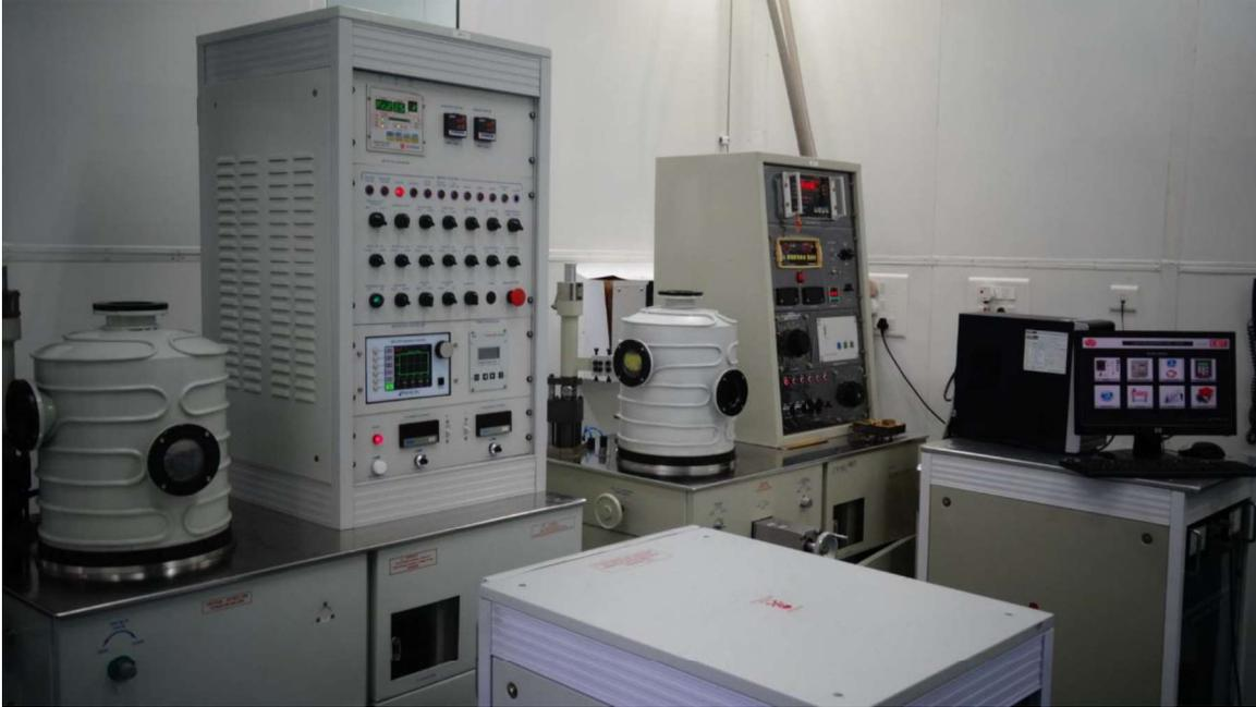
Figure 3.3 Photograph of the thermal and e-beam evaporation system that are used in this work
