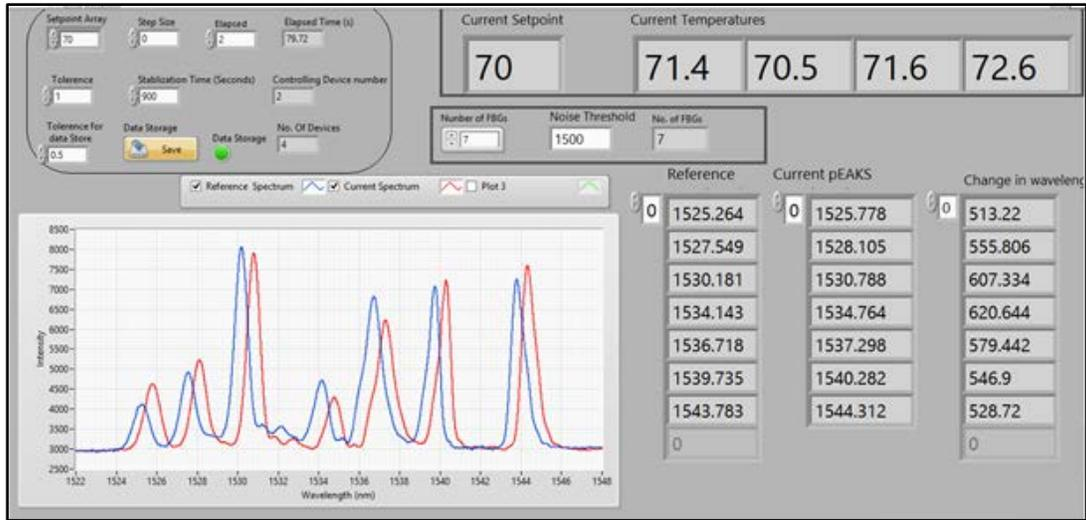
**Fig. 5.15:** Screen shot of the measured wavelength shift and corresponding temperature along the arm of the UHV pump
