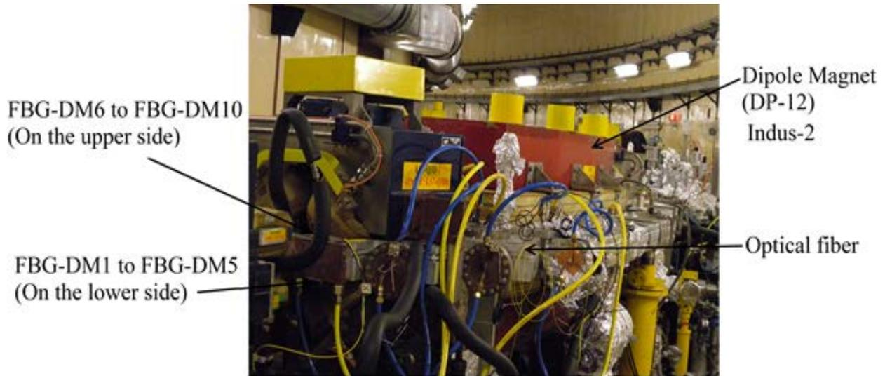
*Fig. 5.19: Experimental arrangement of the distributed temperature monitoring*
