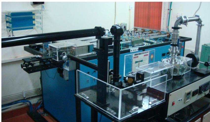
Figure 5.9: A photograph of the deposition set up (based on the laser pyrolysis process).
