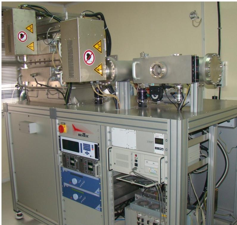
Figure 2.4: A picture of DC magnetron sputtering system, utilized for the deposition of different single and multilayer thin film structure.
