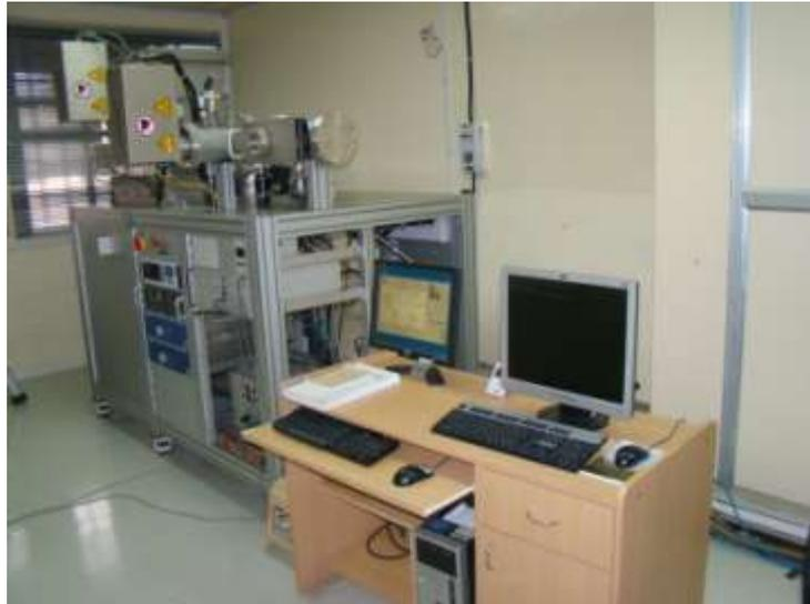
**Figure 2.2** Photograph of magnetron sputtering system in our laboratory used for the fabrication of W/B<sub>4</sub>C multilayer mirrors.
