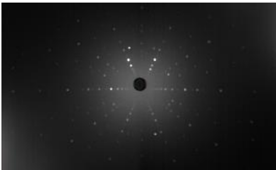
Figure 5.15 Laue pattern of the (100) plane of Nd:GdVO 4 crystal
