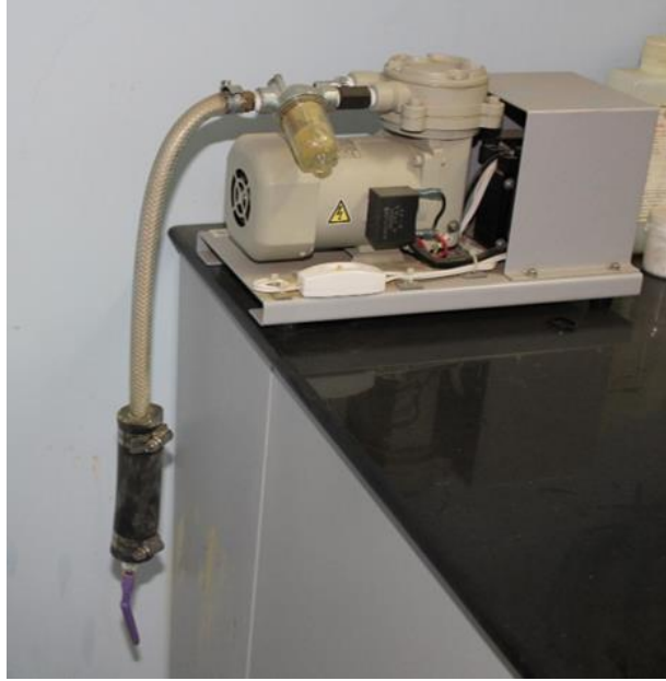
Figure 3.8 Rotary pump sucking the air from the packed rod
