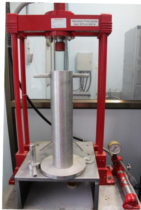
Figure 3.9 Pressing of rod by hydrostatic press system
