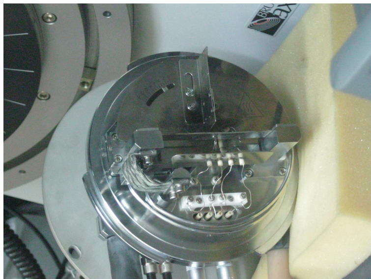
Figure 2.5: Anton Paar high temperature attachment HTK 16.
