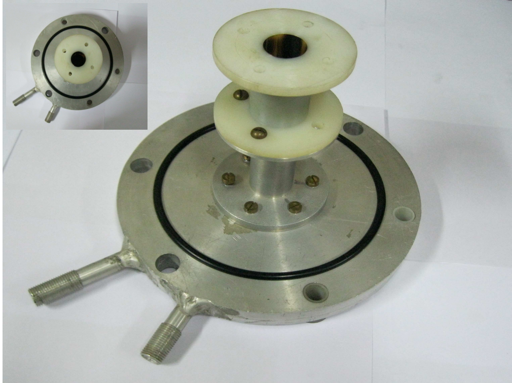
Figure 2.1: The target holder assembly used in the irradiation beamline: the top view of the flange is shown in the inset.
