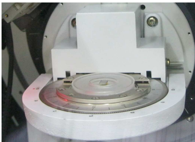
Figure 2.4: Spinner stage for Bruker AXS D8 Advance Diffractometer
