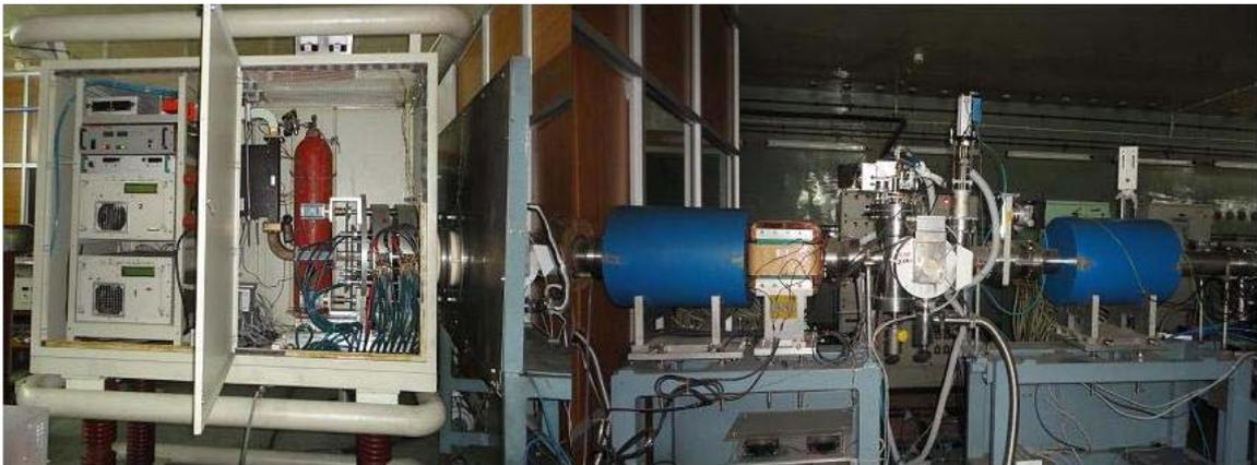
**Fig. 1.1.** 2.45 GHz microwave ion source on the high voltage deck and solenoid based low energy beam transport line.
