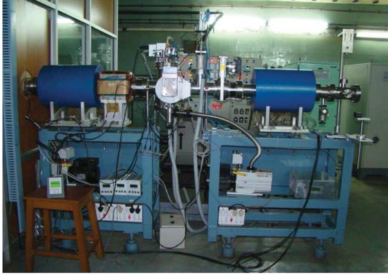
Figure 1.3: *Beam transport line.*
