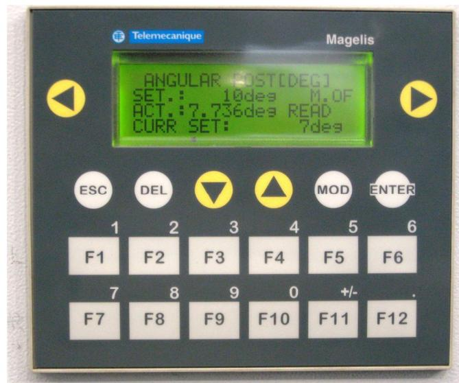
*Figure 6.12: Human machine interface in auto mode.*
