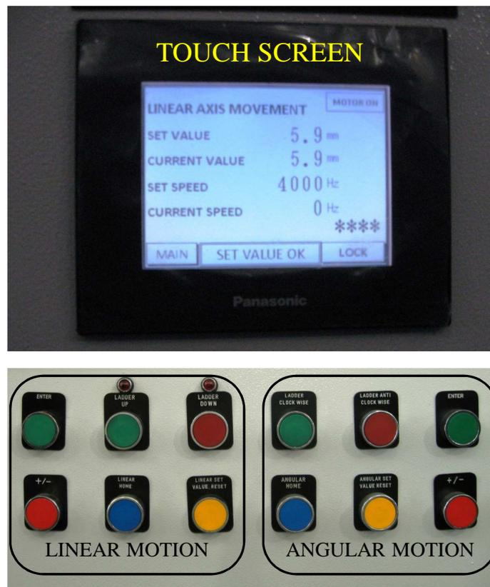
**Figure 6.13:** Human machine interface in manual mode. Details of the buttons are given in the text.
