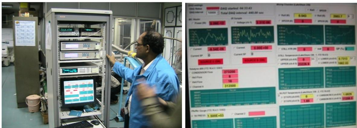
Figure 2.19 Instrumentation rack and Labview based Graphical User Interface for monitoring different parameters of DR
