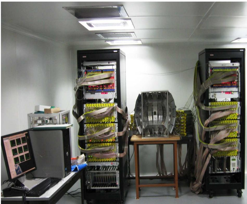
Figure 2.31: Detector array with complete electronics and data acquisition system (DAQ).
