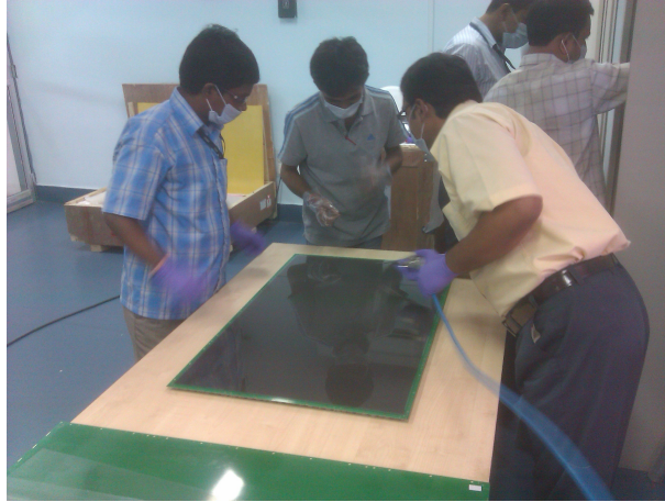
Figure 3.17: Graphite electrode placed on the bottom honeycomb board.
