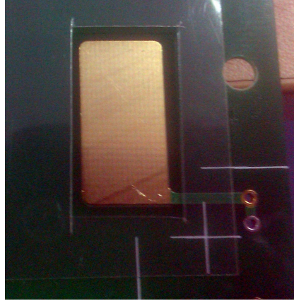
Figure 3.16: New Mylar design with just a small gap for graphite tape.
