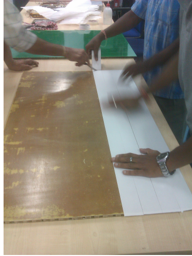
Figure 3.13: Putting the double-sided tape on the honeycomb board before attaching the PCB board to it.
