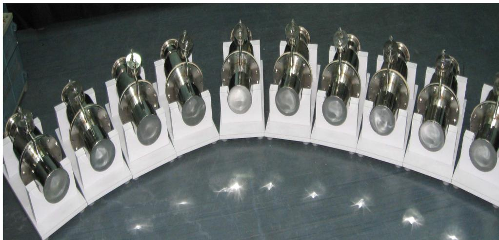
Figure 3.3: *Liquid organic scintillator (BC501A) based neutron time-of-flight detector array.*
