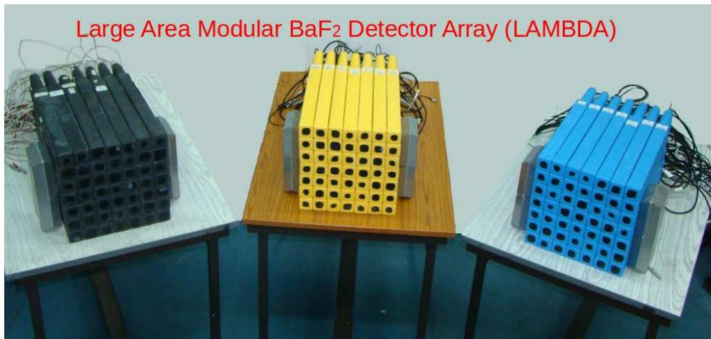
Figure 3.1: *The LAMBDA spectrometer arranged in three  $7 \times 7$  matrix configurations.*
