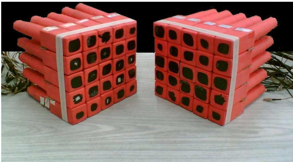
Figure 3.2: The  $\gamma$ -multiplicity filter, split into two blocks of each 25 detectors arranged in  $5 \times 5$  matrix configurations.
