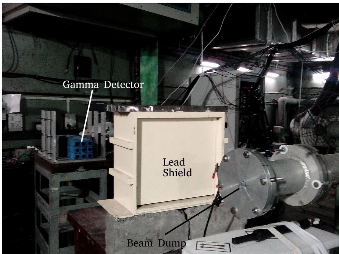
Figure 5.25: Experimental setup for the measurement of photon spectrum. It shows the lead shield and the  $\text{BaF}_2$  detector along with the beam dump position
