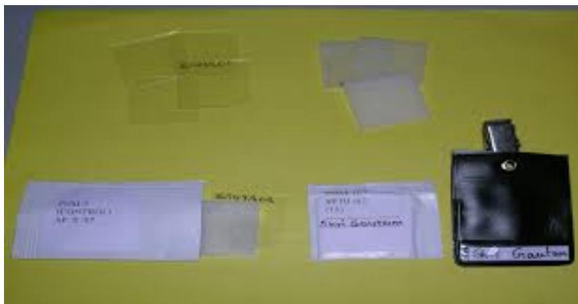
Figure 1.12: CR-39 used for neutron personnel monitoring in India
