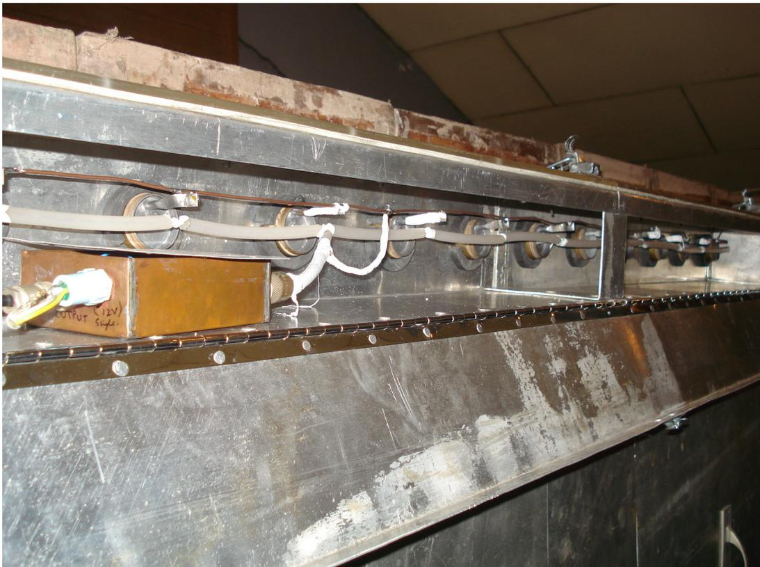
Figure 3.2: Photograph of LFGNM with  $\text{BF}_3$  detectors
