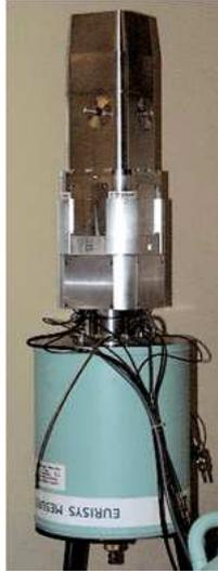
Figure 3.4: Clover HPGe detector at Laboratory.
