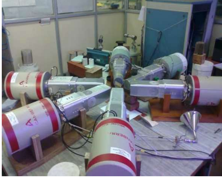
Figure 3.24: Experimental setup at VECC used for the measurement of \beta -decay end-point energy.
