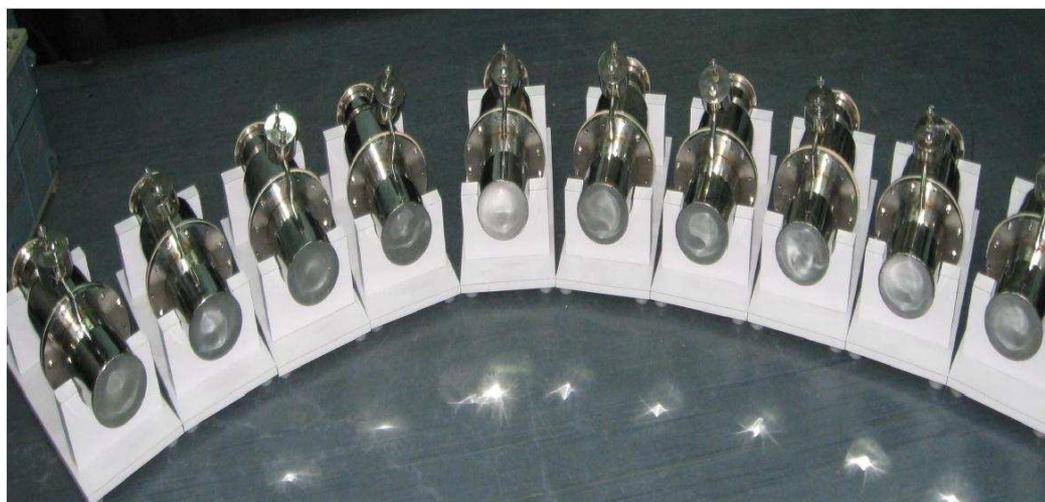
Figure 5.9: *Liquid organic scintillator (BC501A) based neutron TOF array.*
